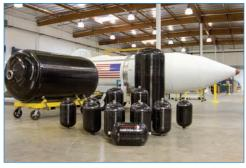
Family of all-composite propellant and pressure tanks
