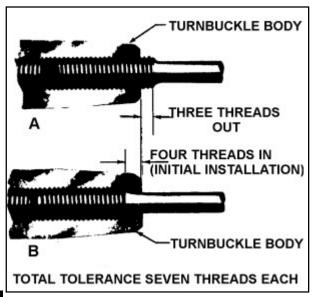
FIGURE 7-25. Turnbuckle thread tolerance.
