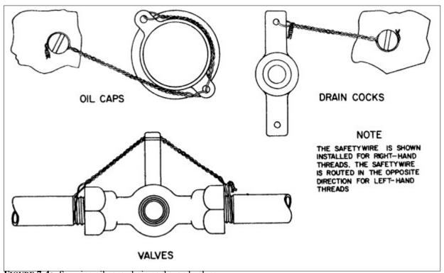
FIGURE 7-4a. Securing oil caps, drain cocks, and valves.
