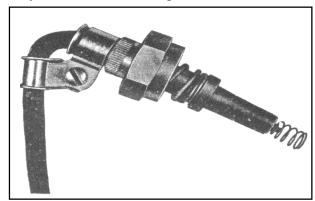
FIGURE 8-8. Typical method of clamping leads.
