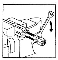
5. Screw nipple into socket using wrench on hex of nipple and leave .005 inches to .031 inches clearance between nipple hex and socket.
