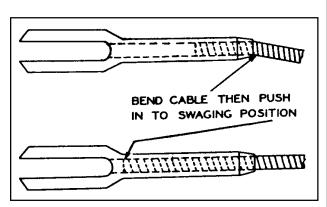
FIGURE 7-10. Insertion of cable into terminal.
