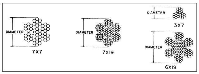
**FIGURE 7-8.** Flexible cable cross section.
