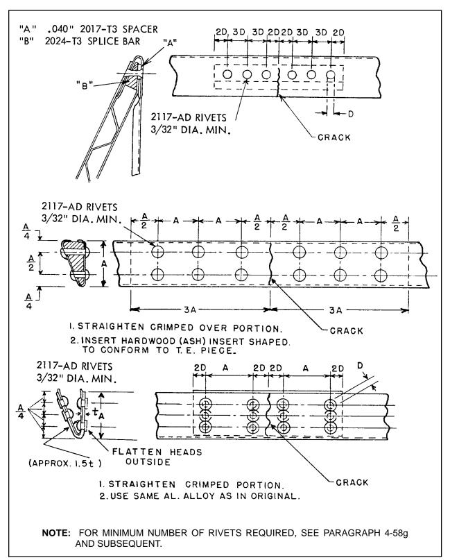
FIGURE 4-15. Typical repairs of trailing edges.
