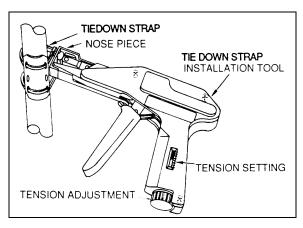
FIGURE 11-30. Tie-down strap installation tool.
