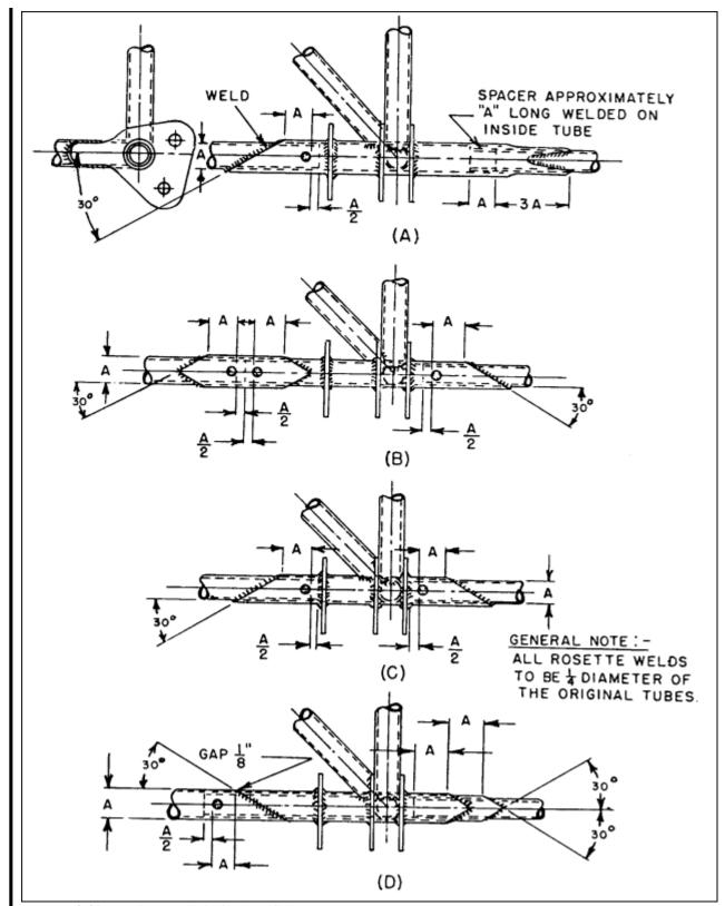
FIGURE 4-41. Repairs at built-in fuselage fittings.
