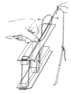
Step 10. After all slack is removed by pulling cord section "D," switch hands and place a thumbnail on the loose knot formed on the right-hand side, then secure the knot by pulling firmly perpendicular to the fabric surface on cord section "E."
