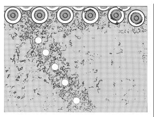
FIGURE 6-8. Filiform corrosion.
