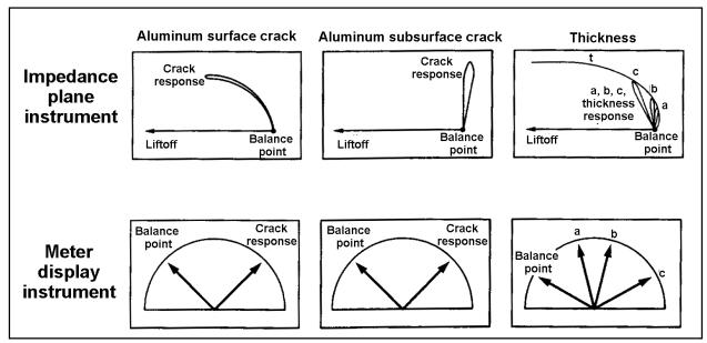
FIGURE 5-5. Typical instrument displays.
