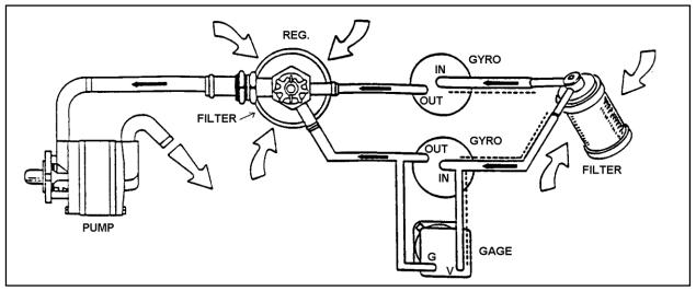
FIGURE 12-3. Instrument vacuum system using a dry-type air pump.
