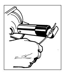
FIGURE 11-34. Shrinking marker on wire.
