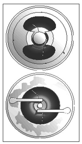
**FIGURE 8-6c.** Typical spark plug with cracked core nose.
