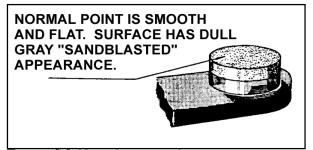
FIGURE 8-9. Normal contact point.
