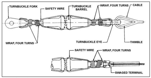
FIGURE 7-27. Securing turnbuckles.
