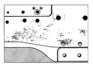
**FIGURE 6-5(a).** Pitting corrosion (external view).
