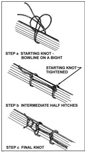
FIGURE 11-16. Double cord lacing.
