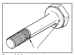
FIGURE 9-2. Typical bolt cracks.
