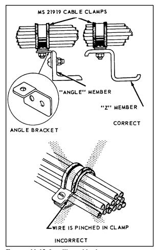
FIGURE 11-13. Installing cable clamp to structure.
