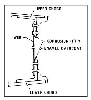
FIGURE 6-13. Fretting corrosion.
