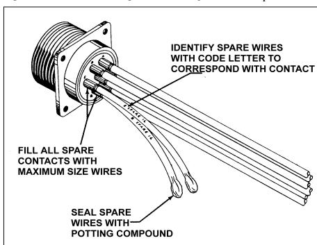
FIGURE 11-38. Spare wires for potting connector.
