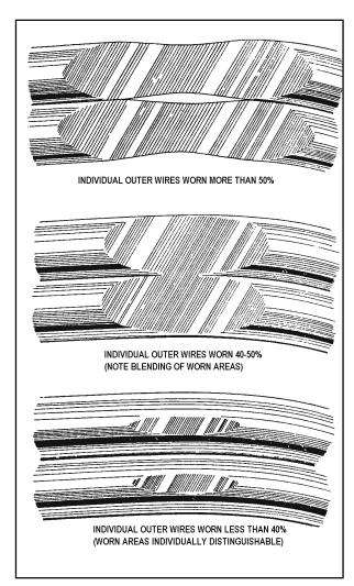
FIGURE 7-17. Cable wear patterns.
