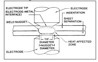
**FIGURE 4-31.** In spot welding, heat is produced by electrical resistance between copper electrodes. Pressure is simultaneously applied to electrode tips to force metal together to complete fusing process. Spot-weldnugget size is directly related to tip size.
