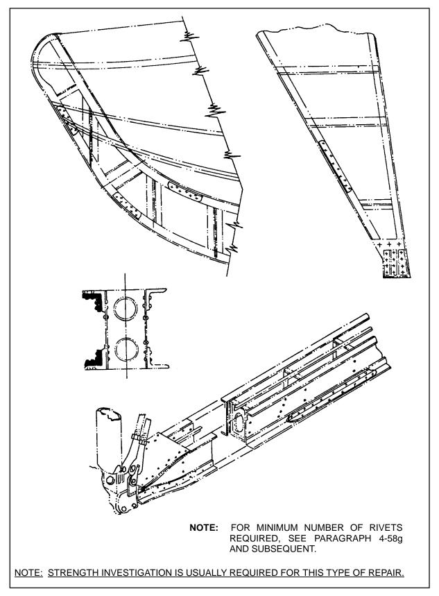
FIGURE 4-19. Application of typical flange splices and reinforcement.
