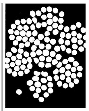
FIGURE 7-19. Internal end view of cable wear.
