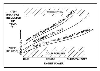
FIGURE 8-2. Chart of spark plug temperature ranges.
