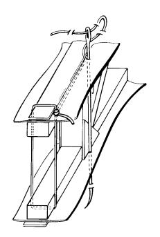
Step 4. Route the needle back thru the exit hole and thru the opposite fabric surface leaving approximately a 3" loop around a finger on the top surface.
