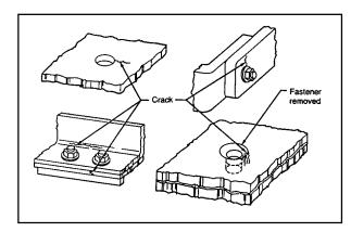
FIGURE 5-6. Typical surface cracks.
