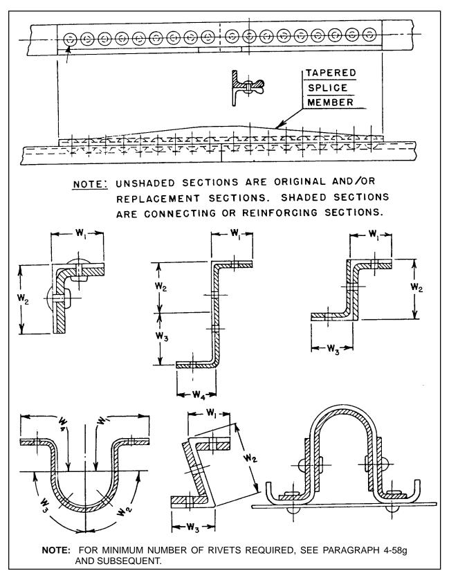
FIGURE 4-17. Typical stringer and flange splices.
