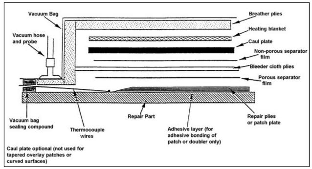
**FIGURE 3-9.** Sample bagging layup cross section.
