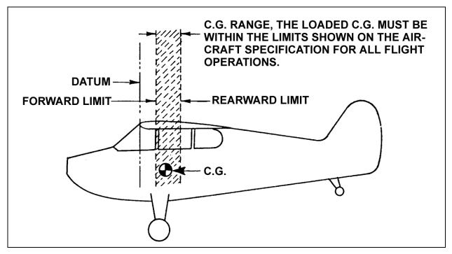
FIGURE 10-7. Operating center of gravity range.
