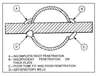
**FIGURE 4-26.** Common defects to avoid when fitting and welding aircraft certification cluster.
