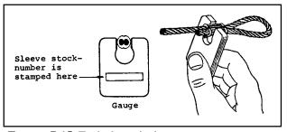
FIGURE 7-15. Typical terminal gauge.
