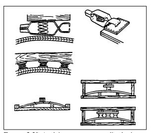
FIGURE 3-20. Applying pressure to acrylic plastics.
