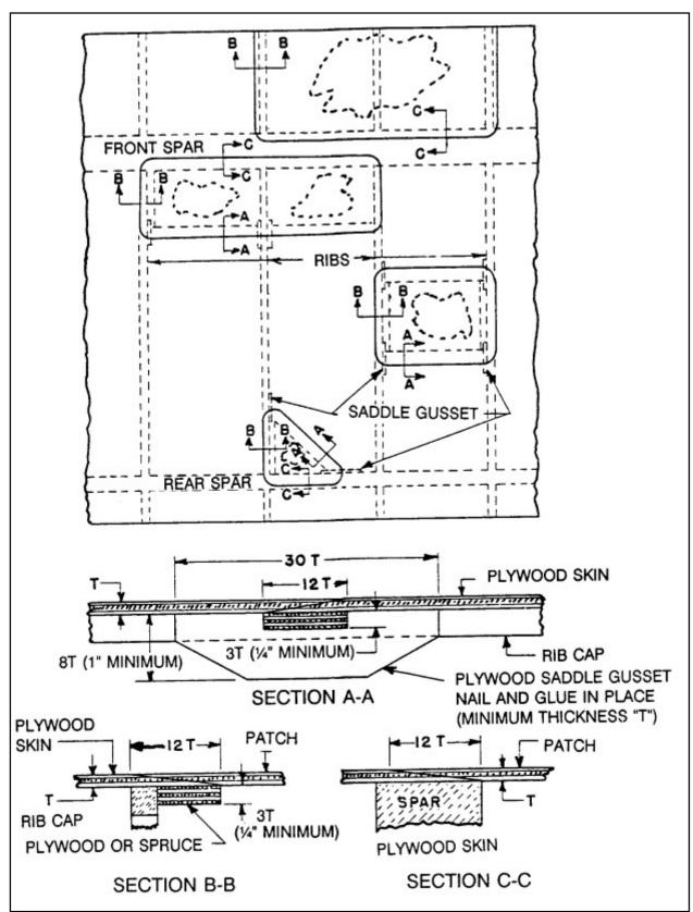
FIGURE 1-16. Scarf patches (back of skin not accessible).
