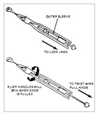
**FIGURE 7-4.** Use of a typical wire twister.
