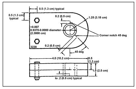
FIGURE 5-20. Example of a typical reference standard.
