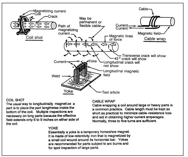
FIGURE 5-12. Longitudinal magnetization.
