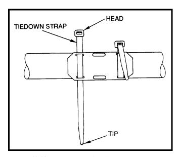
FIGURE 11-29. Tie-down strap installation.
