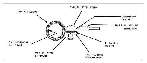
FIGURE 11-22. Aluminum jumper connection to tubular structure.
