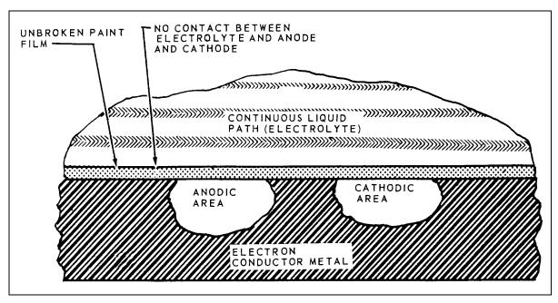
FIGURE 6-2. Elimination of corrosion by application of an organic film to metal surface.
