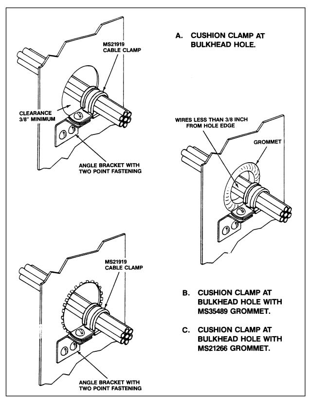
FIGURE 11-14. Clamping at a bulkhead hole.
