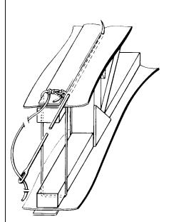
Step 3. Route the needle back thru the right hand hole and exit at the next pre-punched lacing location.
