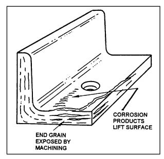
FIGURE 6-10. Exfoliation corrosion.
