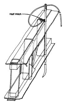
Step 11. After completing all lacing in the same sequence, the end is secured with a half hitch after the modified seine knot. The knot is pulled to the inside by routing the needle thru the wing before cutting the cord to leave the end inside.
