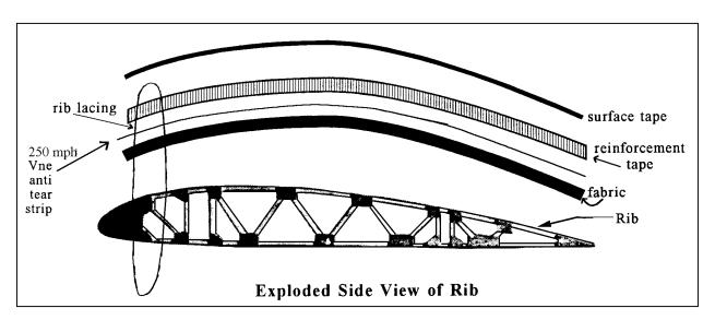
FIGURE 2-3. Exploded side view of rib.
