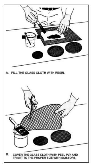
**FIGURE 3-4.** Preparing the fiberglass sandwich.
