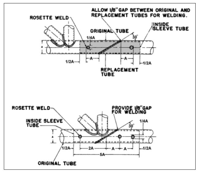
FIGURE 4-37. Splicing by inner-sleeve method.
