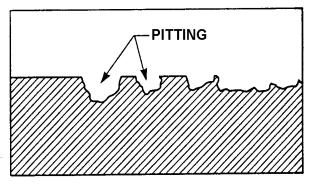
**FIGURE 6-5(b).** Pitting corrosion (magnified cross section).
