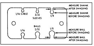
FIGURE 7-13. Typical terminal gauge.
