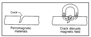
FIGURE 5-9. Magnetic field disrupted.
