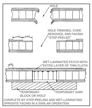
**FIGURE 3-3.** Typical stepped joint repair.
