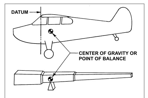
The entire aircraft weight may be considered to be concentrated at the center of gravity. Therefore, the moment of the aircraft about the datum is the weight of the aircraft times the horizontal distance between the C.G. and the datum.
