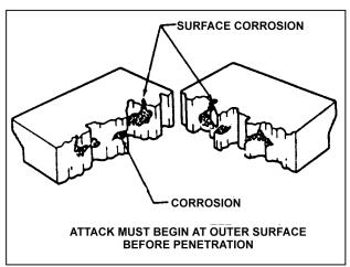
FIGURE 6-3. Corrosion attack.
