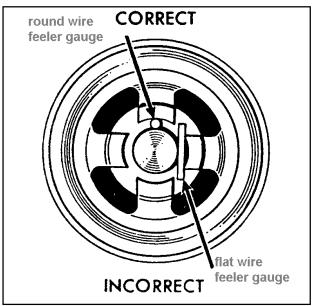
FIGURE 8-5. Method of checking spark plug gap.
