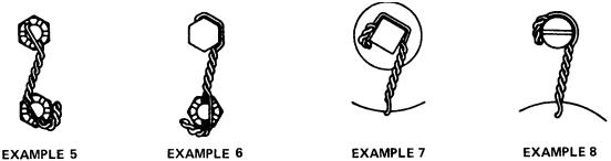
Examples 5, 6, 7, & 8 show methods for wiring various standard items, NOTE: Wire may be wrapped over the unit rather than around it when wiring castellated nuts or on other items when there is a clearance problem.
