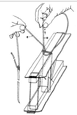
Step 9. Pull cord section "D" perpendicular to the fabric surface to remove all slack in the cord back to the last rib lacing knot while working the loose knot to the right side. Do not pull cord section "E."
