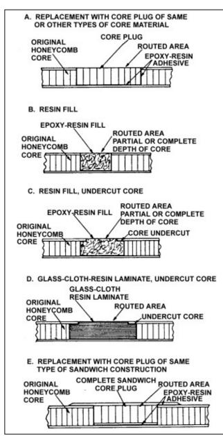
FIGURE 3-10. Typical types of core replacement.
