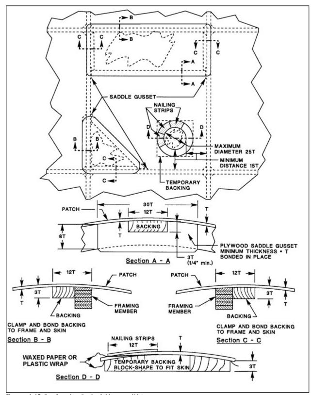
FIGURE 1-15. Scarf patches (back of skin accessible).
