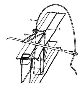
Step 6. The needle tip is routed under cord section "B" to hook and pull cord section "A" aft.
