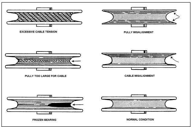
FIGURE 7-20. Pulley wear patterns.
