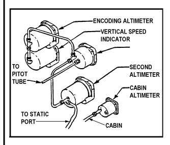
Figure 12-5. Pitot/static system for a small aircraft.
