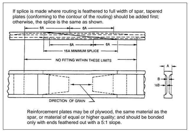
FIGURE 1-6. Method of splicing solid "I" spars.
