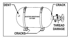
FIGURE 9-14. Oxygen cylinder damage.
