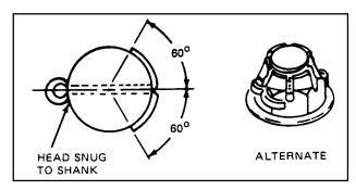
**FIGURE 7-7.** Alternate method for securing with cotter pins.
