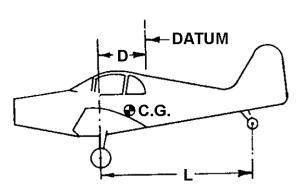
TAIL WHEEL TYPE AIRCRAFT DATUM LOCATED AFT OF THE MAIN WHEELS
