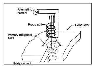
**FIGURE 5-3.** Generating an eddy current.
