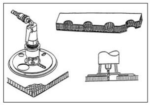
FIGURE 3-13. Honeycomb core removal.
