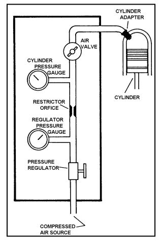
**FIGURE 8-1.** Schematic of differential pressure compression tester.
