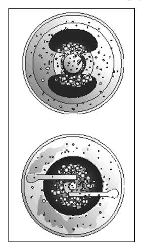
FIGURE 8-6a. Typical lead-fouled spark plug.
