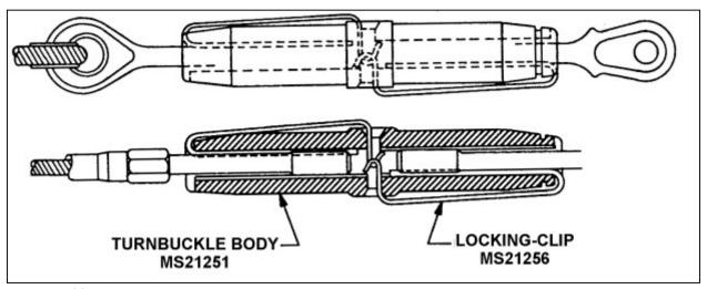
FIGURE 7-28. Clip-type locking device.
