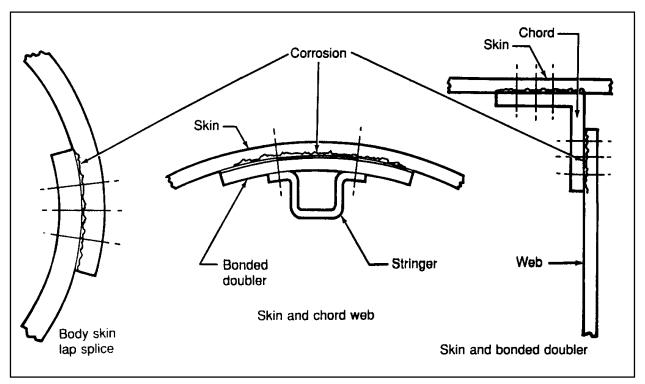
FIGURE 5-8. Typical structural corrosion.
