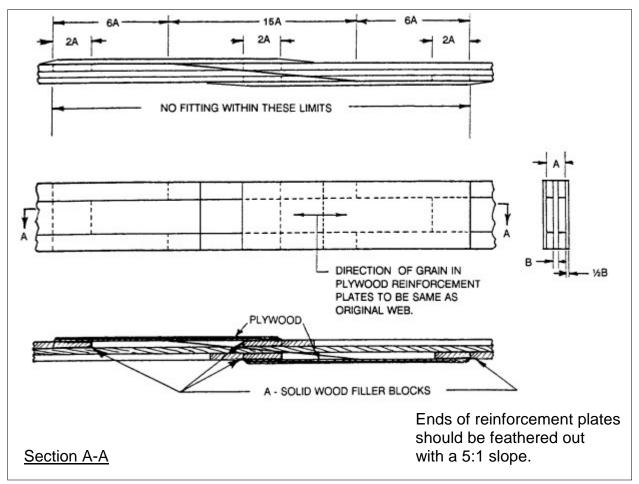
FIGURE 1-7. Repairs to built-up "I" spar.
