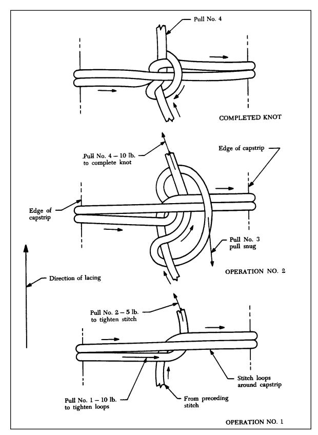
FIGURE 2-7. Standard knot for double-loop lacing.
