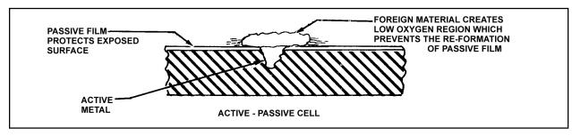
FIGURE 6-7. Active-passive cell.
