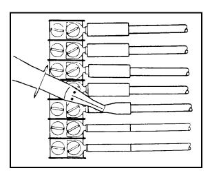
**FIGURE 11-27.** Installation of heat-shrinkable insulation sleeves.
