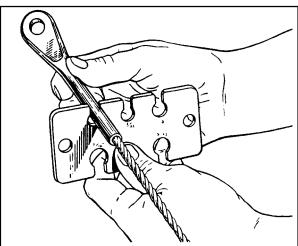
FIGURE 7-11. Gauging terminal shank after swaging.
