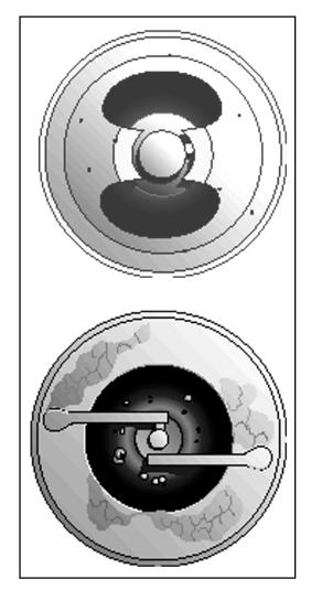
FIGURE 8-6e. Typical spark plug with bridged electrodes.
