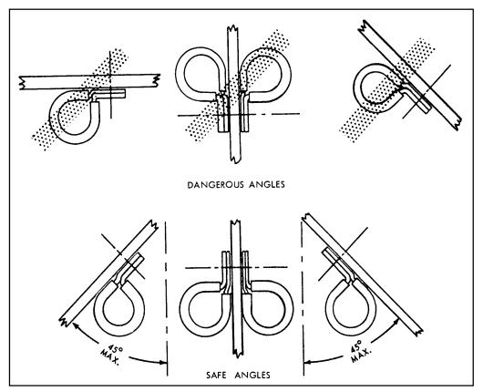
FIGURE 11-11. Safe angle for cable clamps.
