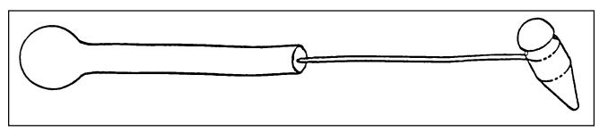
FIGURE 5-22. Sample of special tap hammer.
