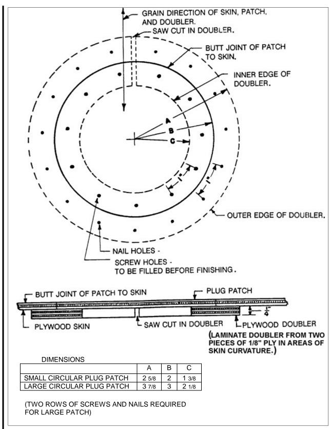
FIGURE 1-18. Round plug patch assembly.
