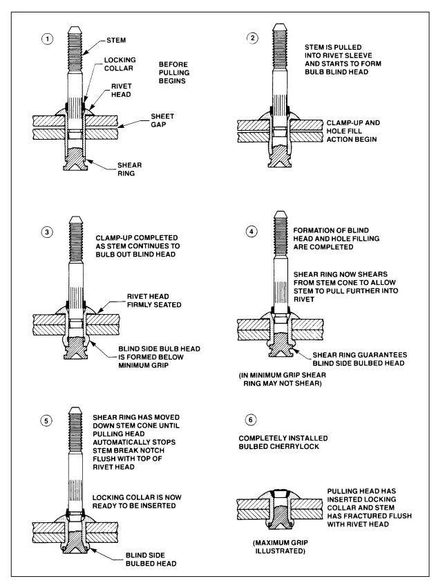
FIGURE 4-8. Mechanical-lock (Bulbed Cherrylock) Cherry rivet.
