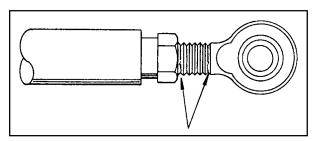
FIGURE 9-5. Typical rod-end cracks.
