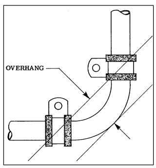
**FIGURE 8-12.** Location of clamps at tube bends.
