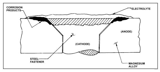
FIGURE 6-11. Galvanic corrosion of magnesium adjacent to steel fastener.
