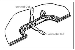
FIGURE 3-15. Removal of core with core knife.
