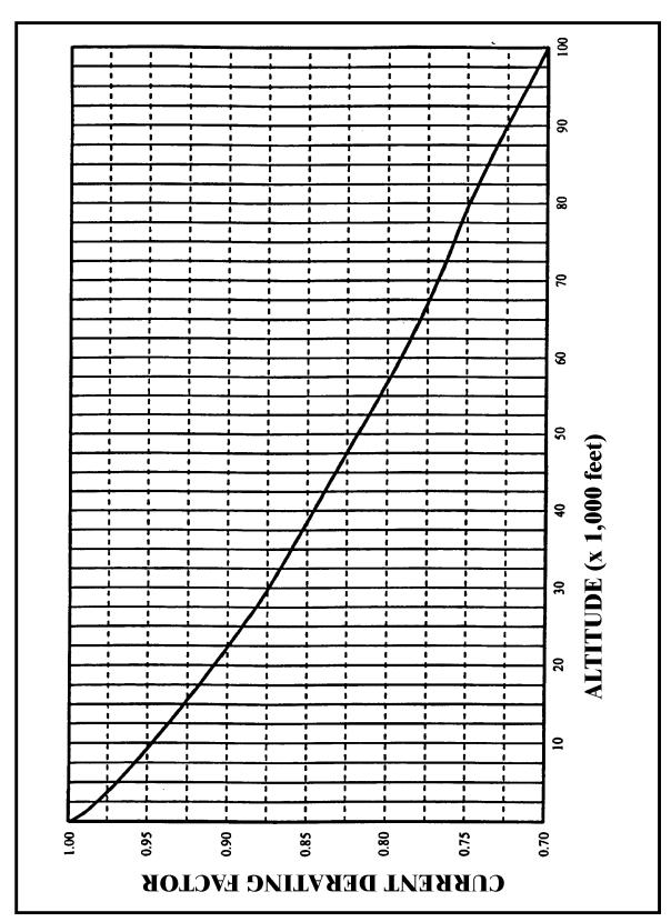
FIGURE 11-6. Altitude derating curve.
