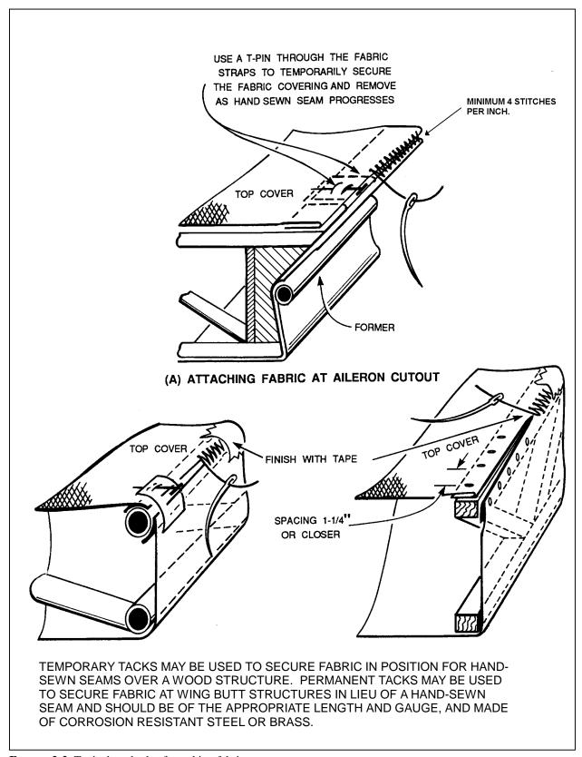
**FIGURE 2-2.** Typical methods of attaching fabric.
