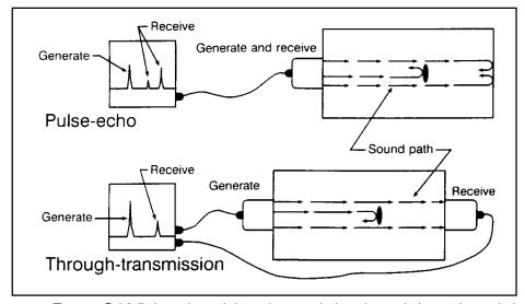
FIGURE 5-16. Pulse-echo and through-transmission ultrasonic inspection techniques.
