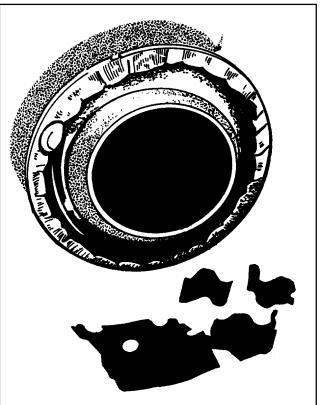
FIGURE 8-18. Loose pieces of a failed internal baffle.
