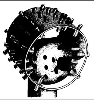
**FIGURE 8-17.** Section of a muffler showing typical internal baffle failure.
