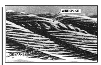
FIGURE 7-22. Manufacturer's wire splice.
