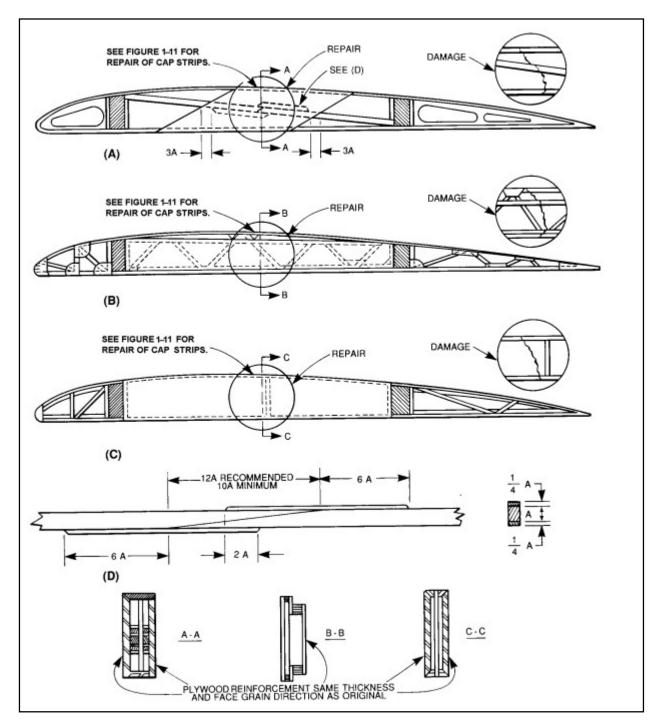
**FIGURE 1-12.** Typical wing compression rib repairs.
