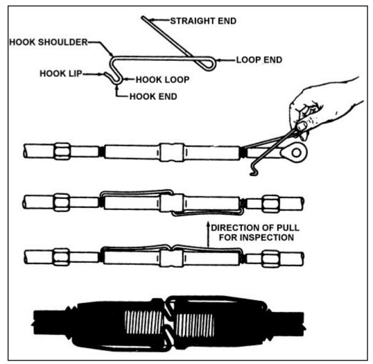
FIGURE 7-27. Assembling and securing clip-locking turnbuckles
