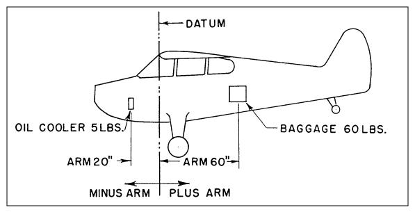
FIGURE 10-2. Illustration of arm (or moment arm).
