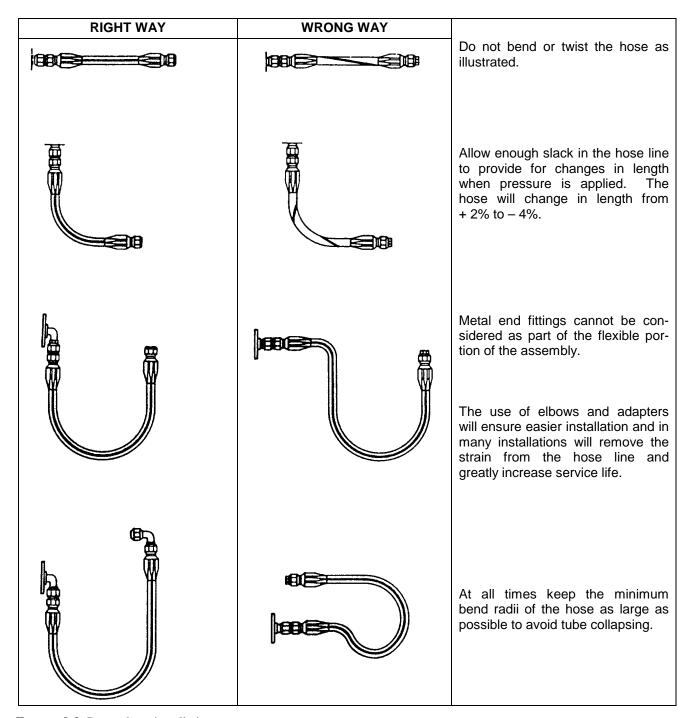
**FIGURE 9-9.** Proper hose installations.
