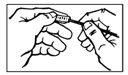
FIGURE 11-33. Inserting wire into marker.
