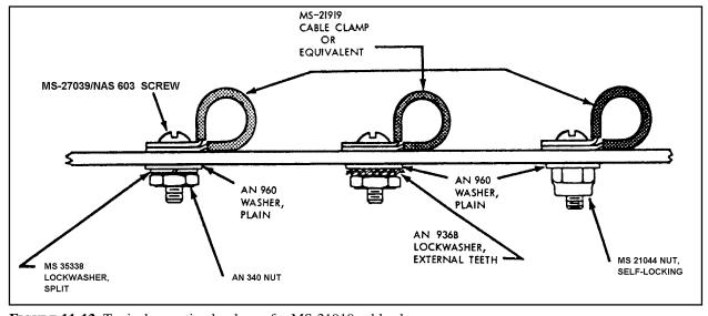
FIGURE 11-12. Typical mounting hardware for MS-21919 cable clamps.
