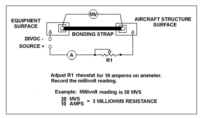
Figure 11-19. Millivolt drop test.
