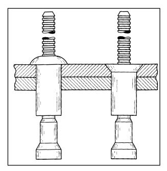
FIGURE 4-7. Self plugging friction-lock Cherry rivets.
