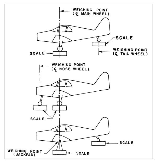
FIGURE 10-8. Weighing point centerline.
