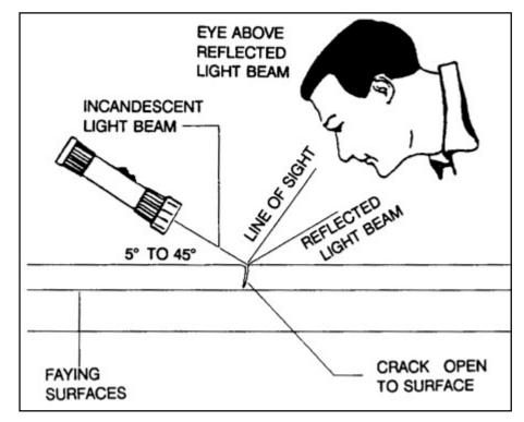
FIGURE 5-2. Using a flashlight to inspect for cracks.
