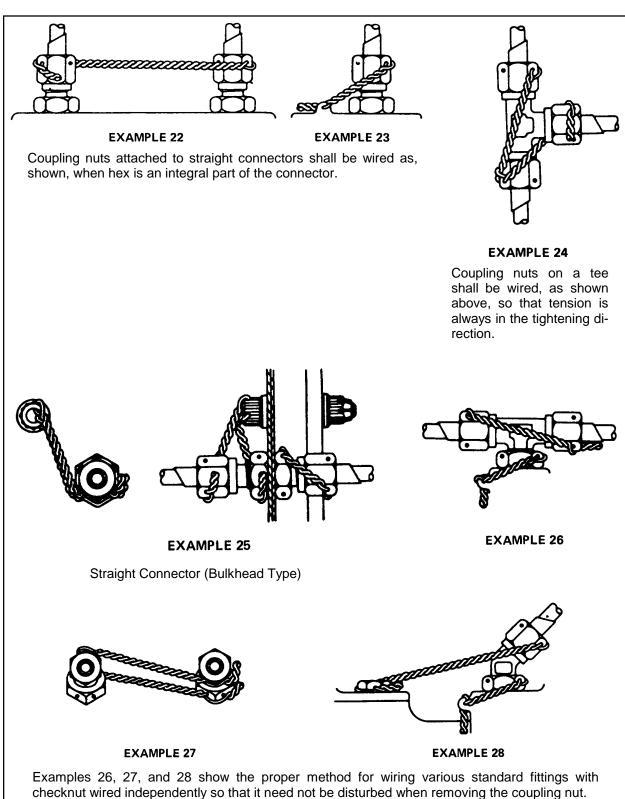
**FIGURE 7-5b.** Safety-wiring procedures.
