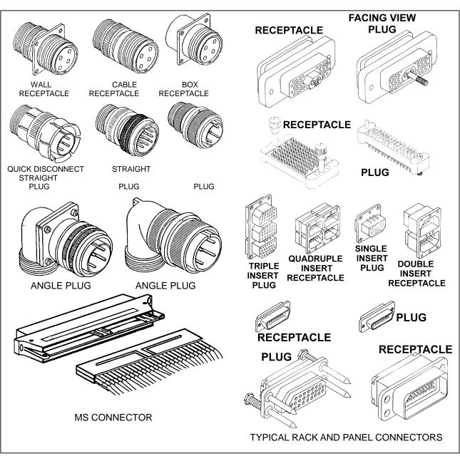
FIGURE 11-36. Different types of connectors.
