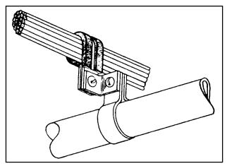
FIGURE 11-10. Separation of wires from plumbing lines.
