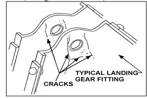
FIGURE 9-3. Typical cracks near bolt holes.
