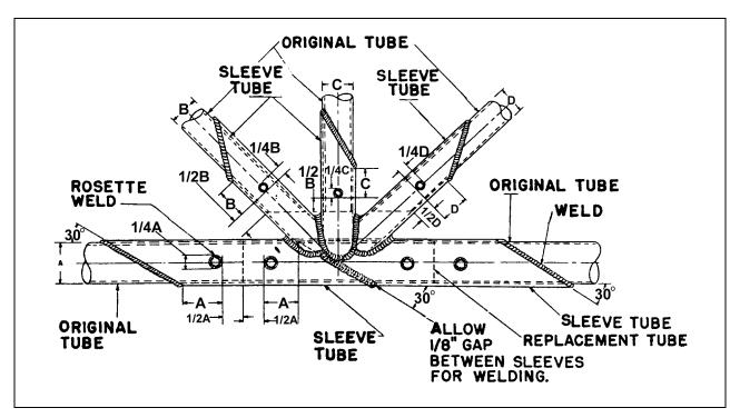
FIGURE 4-39. Tube replacement at a station by welded outer sleeves.
