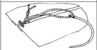
**Step 2.** Start the stitch by routing through the loop, positioning the square knot on the inside.
