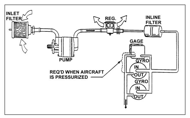
FIGURE 12-4. Instrument pressure system using a dry-type air pump.
