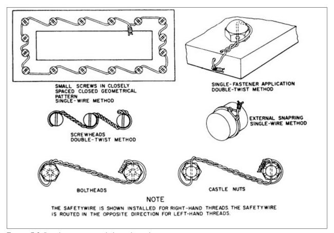
FIGURE 7-3. Securing screws, nuts, bolts, and snaprings.
