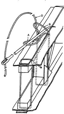
Step 7. The needle tip is then routed over the top of cord section "A" and under cord section "B."
