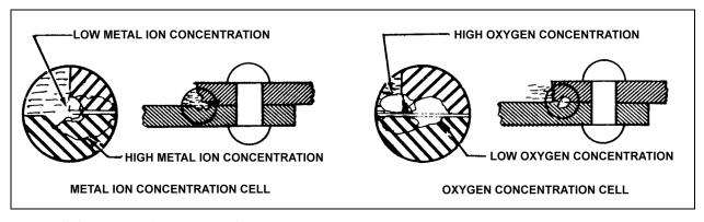
FIGURE 6-6. Concentration cell corrosion.
