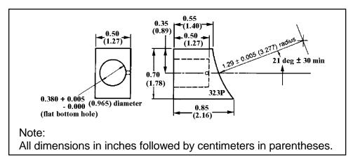
FIGURE 5-18. Example of position fixture and shoe.
