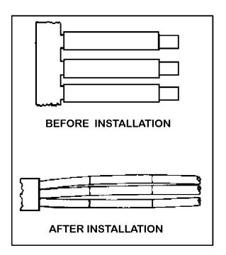
FIGURE 11-26. Standard sleeves (135 °C).
