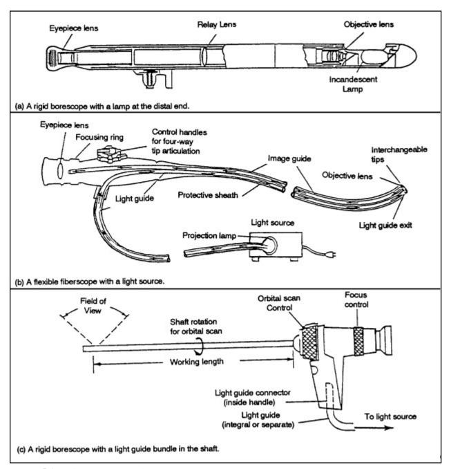
**FIGURE 5-1.** Typical borescope designs.
