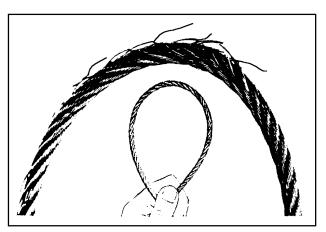
**FIGURE 7-16.** Cable inspection technique.
