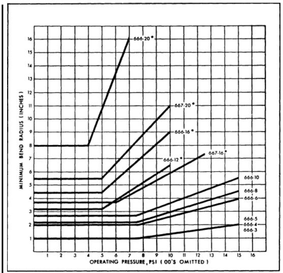
Figure 9-12. Minimum bend radii—Teflon hose.
