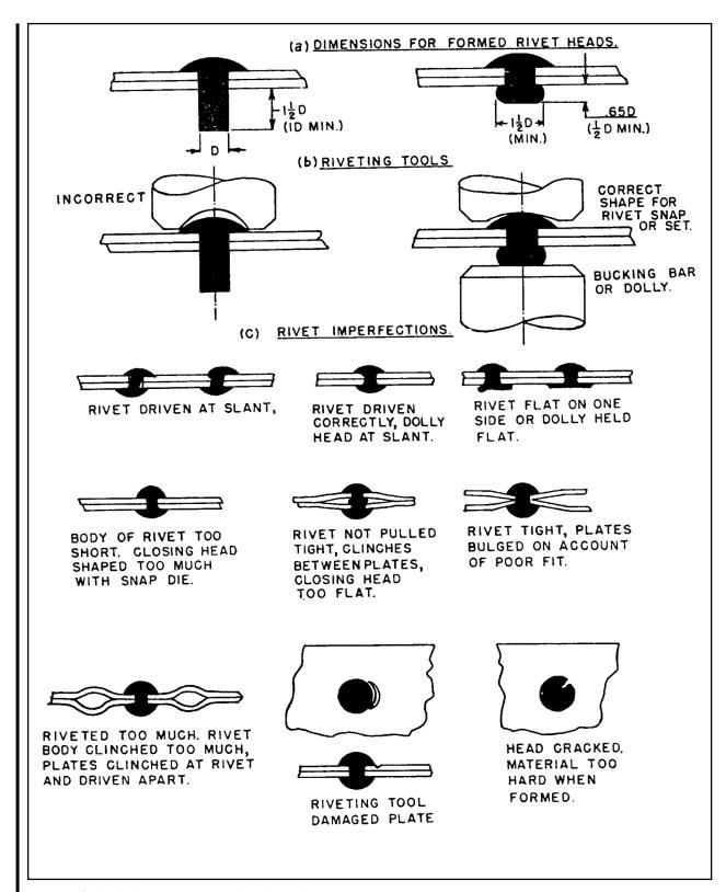
FIGURE 4-6. Riveting practice and rivet imperfections.
