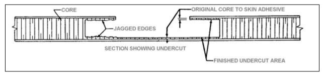
FIGURE 3-11. Typical undercut core material cavity.
