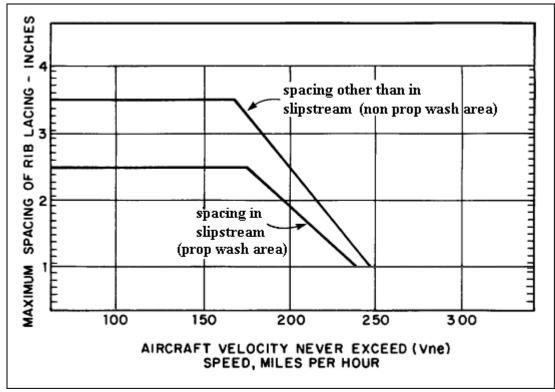
FIGURE 2-12. Fabric attachment spacing
