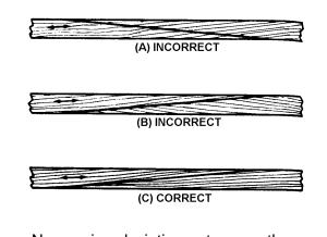
No grain deviation steeper than 1 in 15 should be present in an outer eighth of the depth of the spar. In adjacent eighths, deviations involving steeper slopes, such as a wave in a few growth layers, are unlikely to be harmful. Local grain slope deviations in excess of those specified may be permitted in spar flanges only in the inner one-fourth of the flange depth.
