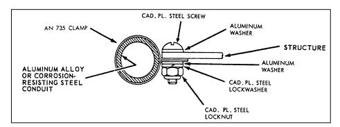
FIGURE 11-21. Bonding conduit to structure.
