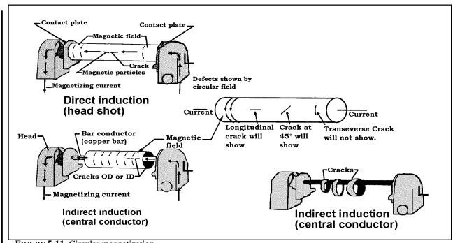
FIGURE 5-11. Circular magnetization.
