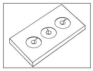
FIGURE 9-4. Typical bolt hole cracks.
