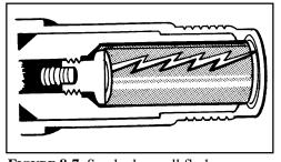
FIGURE 8-7. Spark plug well flashover.
