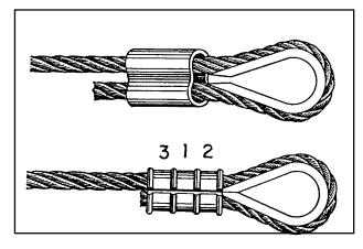
**FIGURE 7-14.** Typical thimble-eye splice.
