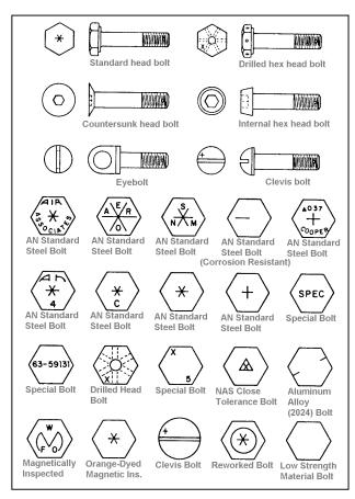
FIGURE 7-1. Typical aircraft bolt markings.
