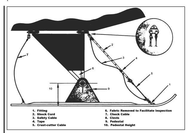
FIGURE 9-1. A typical ski installation.
