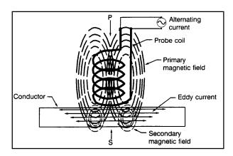
FIGURE 5-4. Detecting an eddy current.
