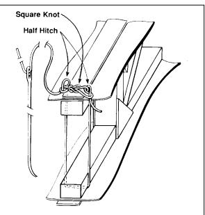
Step 2. Secure the tight square knot with a half hitch at each side.
