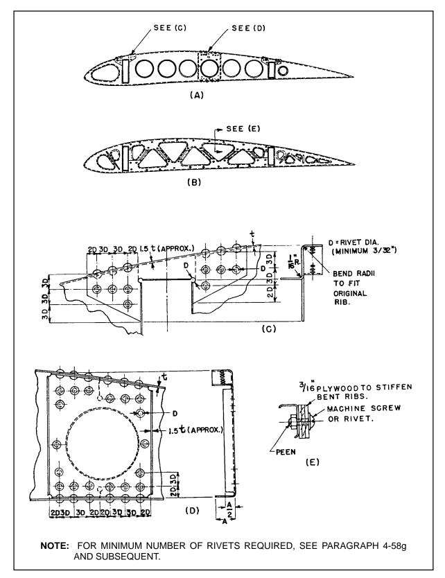
FIGURE 4-14. Typical metal rib repairs (usually found on small and medium-size aircraft).
