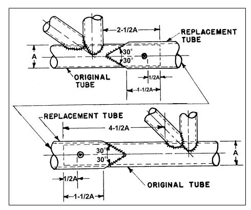
FIGURE 4-40. Splicing using larger diameter replacement tube.
