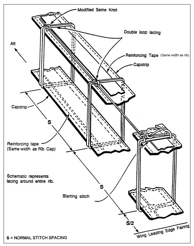
FIGURE 2-8. Standard double-loop lacing (optional).
