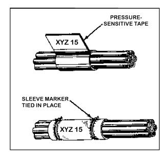
**FIGURE 11-25.** Identification of wire bundles and harnesses.
