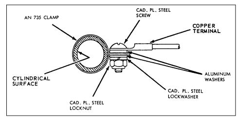
FIGURE 11-20. Copper jumper connector to tubular structure.
