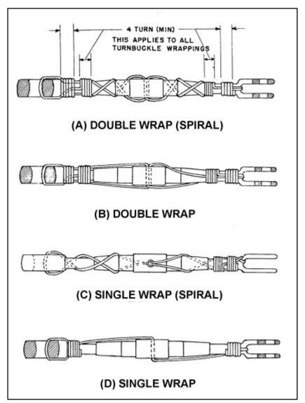
FIGURE 7-26. Safetying turnbuckles.
