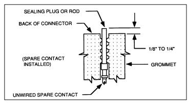
FIGURE 11-40. Sealing unused contact cavities-unpressurized areas-(cut-away view).
