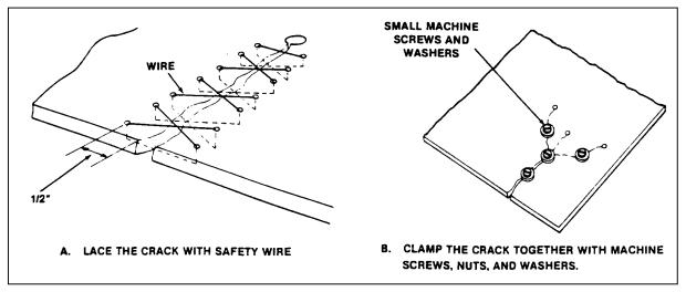
FIGURE 3-24. Temporary repairs to cracked windshields or windows.
