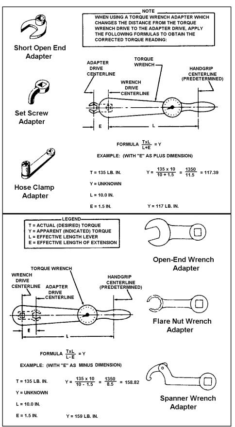
FIGURE 7-2. Torque wrench with various adapters.
