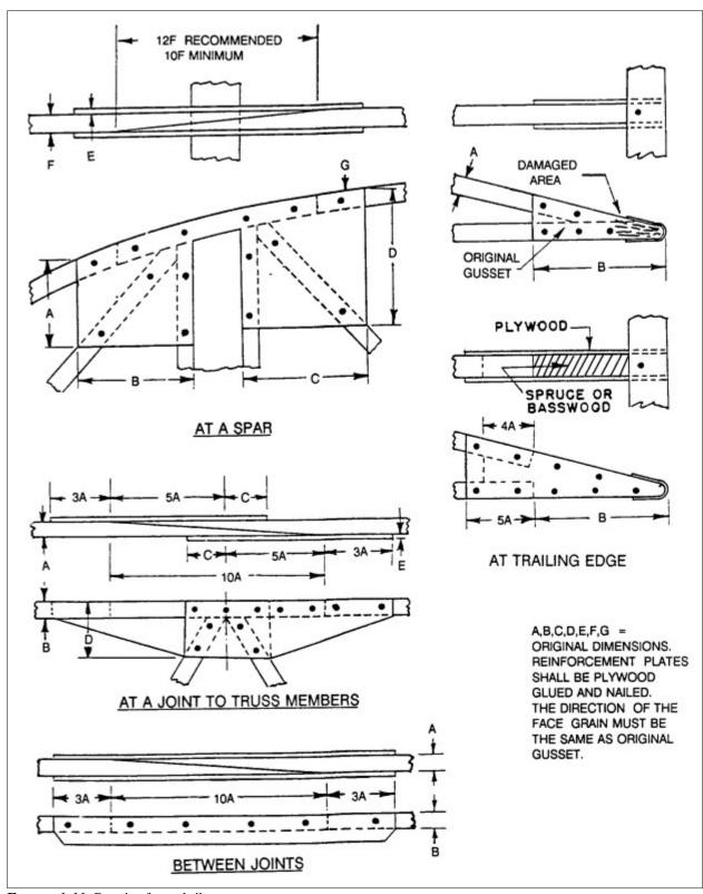
FIGURE 1-11. Repair of wood ribs.
