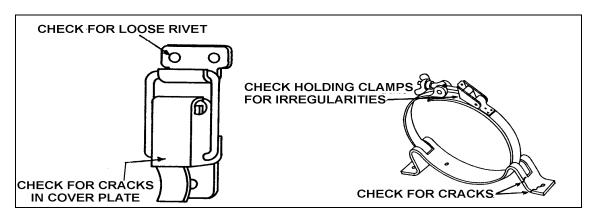
FIGURE 9-15. Cylinder brackets and clamps.
