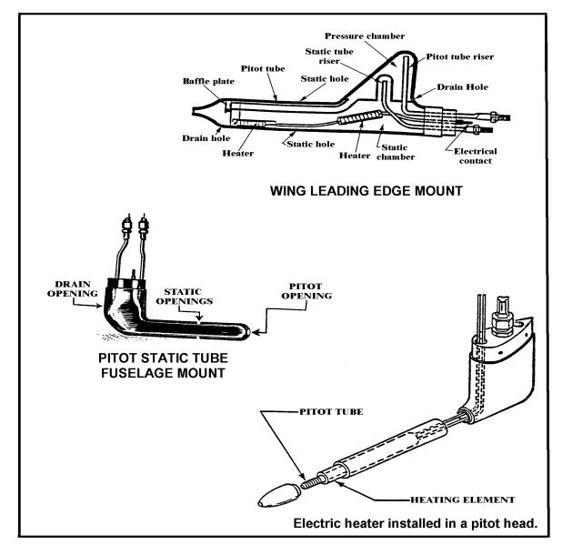
Figure 12-6. Pitot/Static Tube Head
