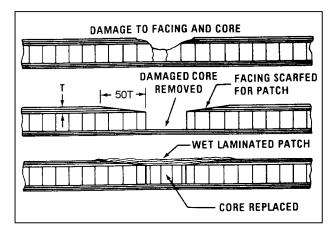
FIGURE 3-2. Typical core and facing repair.
