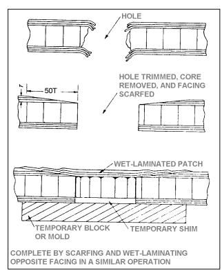
**FIGURE 3-7.** Typical scarf joint repair.
