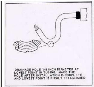
**FIGURE 11-9b.** Drainage hole in low point of tubing.
