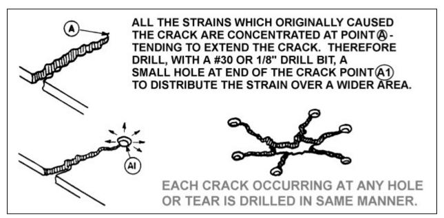
FIGURE 3-21. Stop-drilling cracks.
