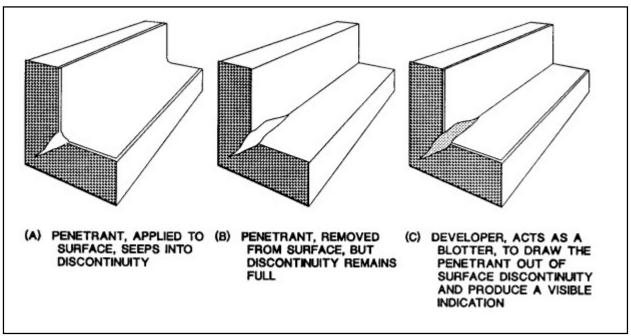
**FIGURE 5-13.** Penetrant and developer action.
