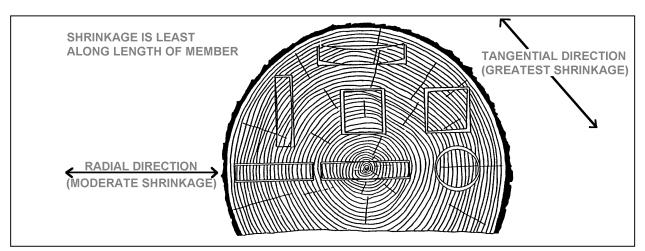
FIGURE 1-1. Relative shrinkage of wood members due to drying.
