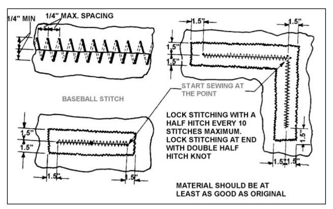
FIGURE 2-13. Repair of tears in fabric.
