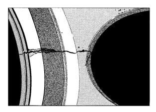
FIGURE 6-12. Stress corrosion cracking.
