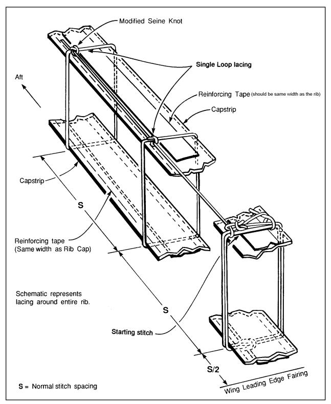
FIGURE 2-6. Standard single-loop lacing.
