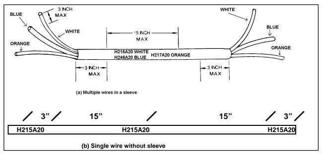
**FIGURE 11-23.** Spacing of printed identification marks (direct marking).
