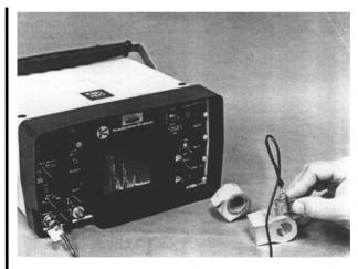
**FIGURE 5-17.** Typical portable ultrasonic inspection instrument.
