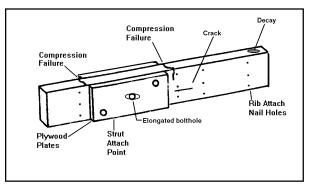
FIGURE 1-3. Likely areas to incur structural damage.
