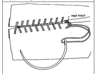
**Step 3.** Complete the hand-stitch and secure the stitching with a half hitch at a maximum each 10 stitches.
