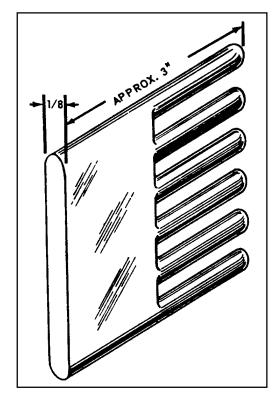
FIGURE 11-8. Comb for straightening wires in bundles.
