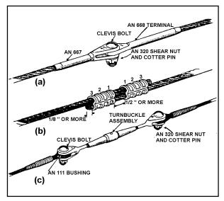
FIGURE 7-12. Typical cable splices.
