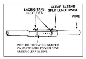
FIGURE 11-32. Temporary wire identification marker.
