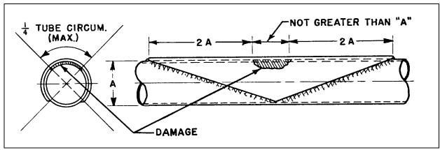
FIGURE 4-36. Welded patch repair.
