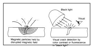
**FIGURE 5-10.** Crack detection by magnetic particle inspection.
