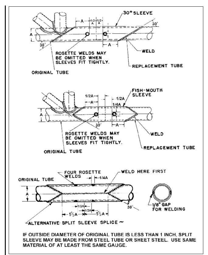
**FIGURE 4-38.** Splicing by outer-sleeve method (replacement by welded outside sleeve).
