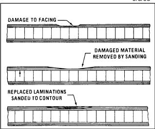
FIGURE 3-1. Typical laminate (facing) repair.
