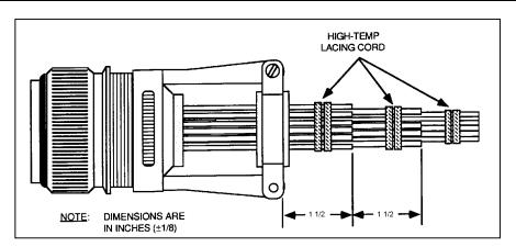
FIGURE 11-39. Stub wire installation.
