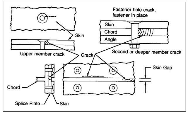
FIGURE 5-7. Typical subsurface cracks.
