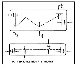
FIGURE 9-13. Repair dimensions.
