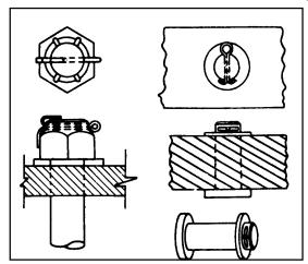
**FIGURE 7-6.** Securing with cotter pins.
