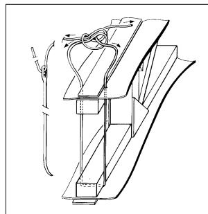
Step 1. Tie a square knot by passing the short end of the cord thru the fold-back loop, as illustrated.
