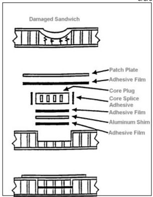
FIGURE 3-16. Details of core repair.
