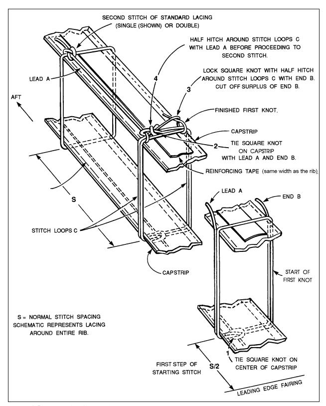
FIGURE 2-5. Starting stitch for rib lacing.
