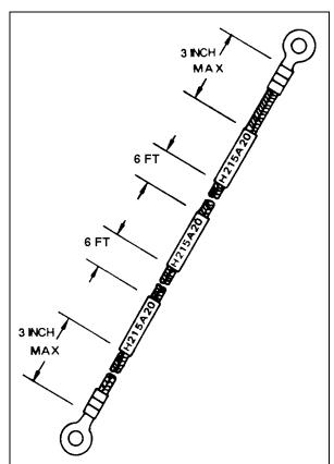
FIGURE 11-24. Spacing of printed identification marks (indirect marking).
