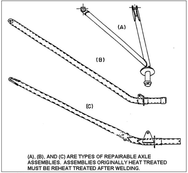
FIGURE 4-46. Representative types of repairable axle assemblies.
