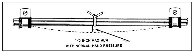
FIGURE 11-9a. Slack between supports
