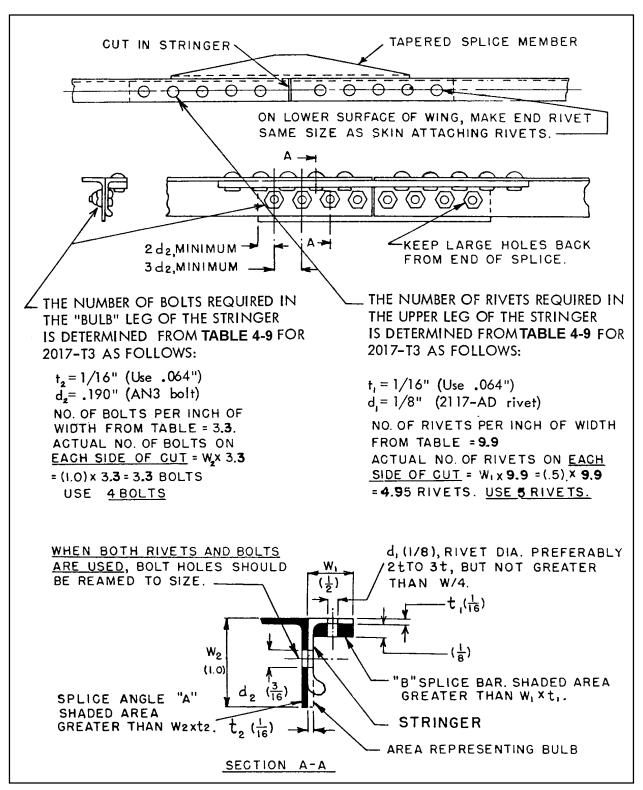
**FIGURE 4-18.** Example of stringer splice (material-2017 alloy).
