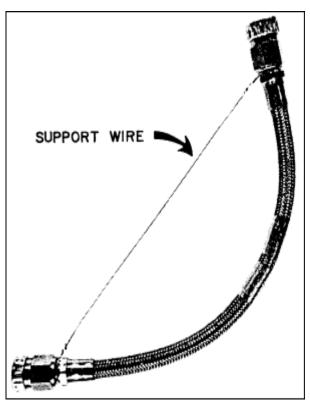
FIGURE 9-11. Suggested handling of preformed hose.
