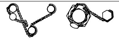
Examples 12 and 13 show methods for attaching lead seal to protect critical adjustments.
