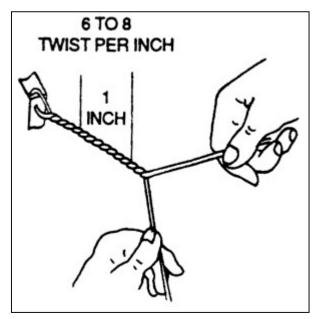
**FIGURE 7-3a.** Wire twisting by hand.
