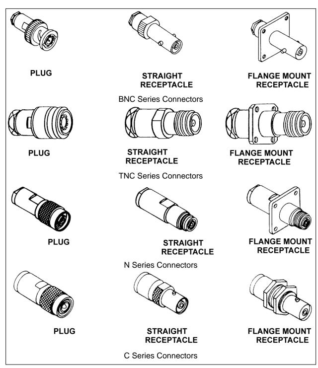
FIGURE 11-37. Coax cable connectors.
