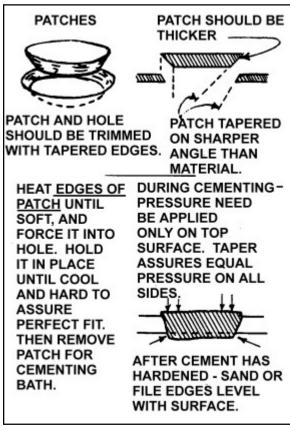
FIGURE 3-23. Plug patch repair.
