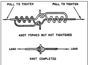
The splice knot is made by crossing the ends of the cord, and making four complete wraps with the small end of the free piece around the end of the standing piece. The end is then doubled back through the formed loop. The other free end is wrapped and doubled back. The long ends of the cords are then pulled until the knot is tight. The short ends are cut close to the knot. This finishes the splice knot.
