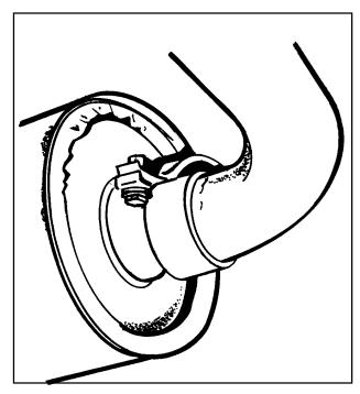
**FIGURE 8-22.** Effect of improperly positioned exhaust pipe/muffler clamp.
