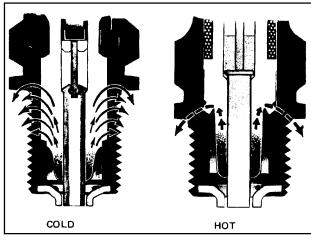
FIGURE 8-3. Hot and cold spark plugs.
