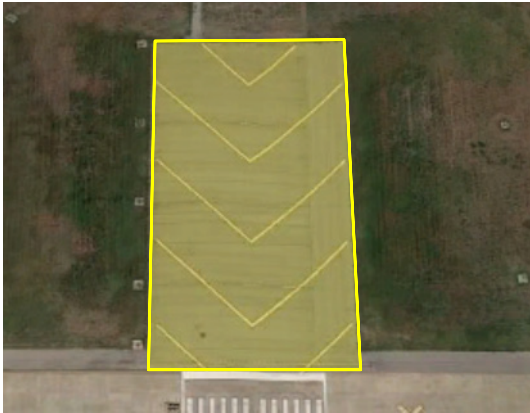
Figure 5-25. Runway Blast Pad
