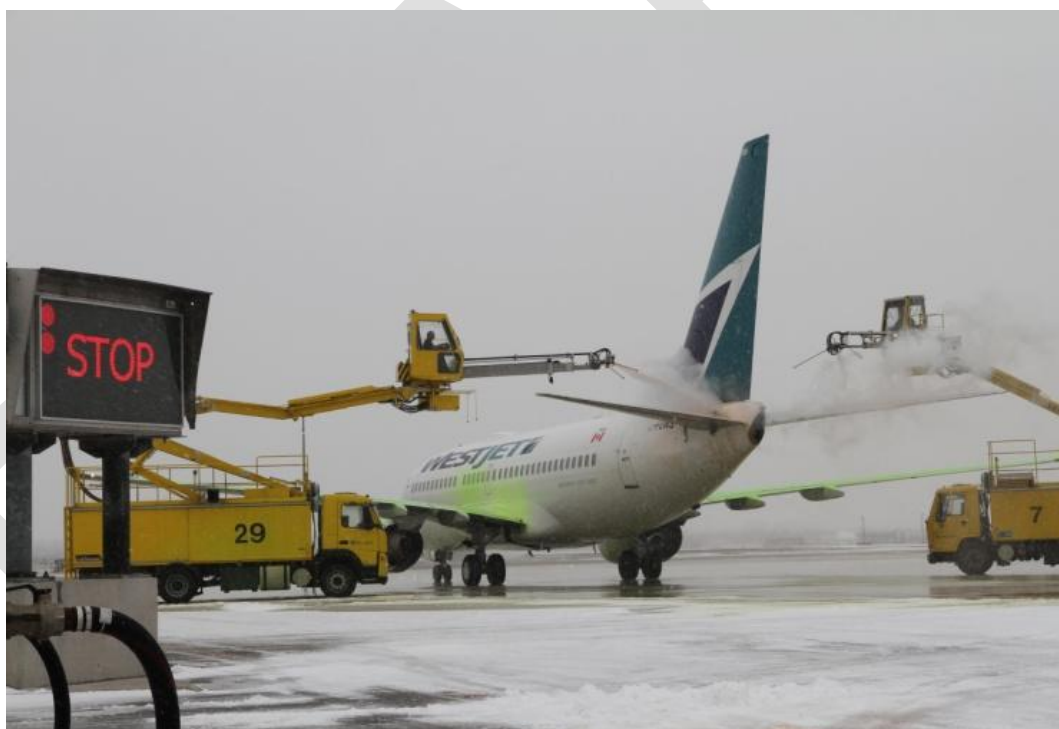
Figure 3-5(b). Electronic message board indicating the aircraft has reached the stop point of the deicing pad
