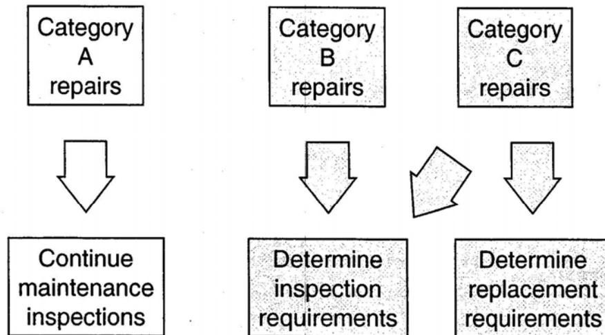
Once a repair has been determined to be Category A, no further work is needed. It can continue to be inspected by normal maintenance.
