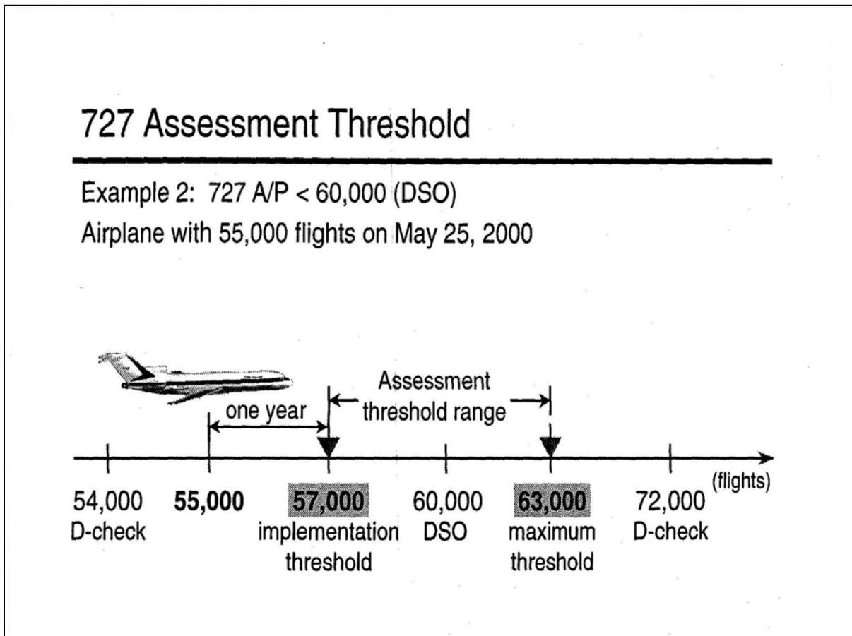
This example is for a 727 airplane with 55,000 flight cycles on May 25, 2000. This was over 45,000 flights (75 percent DSG/DSO), but less than 60,000 flights (DSG/DSO); thus:
