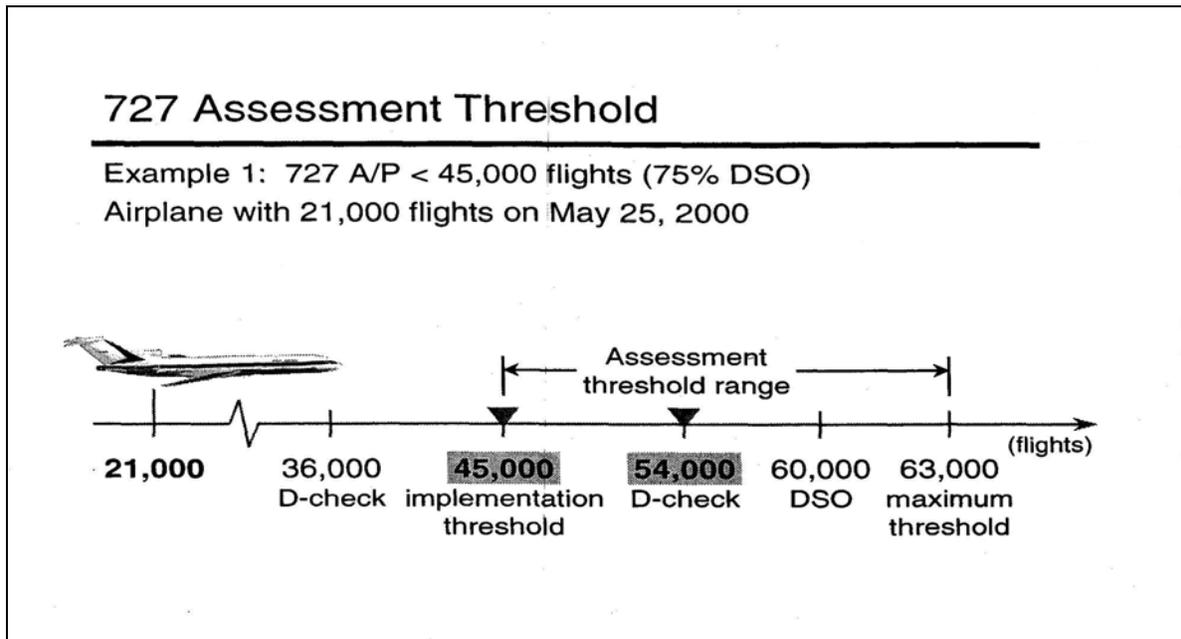
This example is of the implementation and assessment thresholds for a 727 airplane that had 21,000 flight cycles on May 25, 2000. This was less than 45,000 flights (75 percent design service goal (DSG)/design service objective (DSO)); thus:
