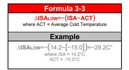
The effective glidepath angle at  $\Delta$ **ISA**LOW ( $\theta_{\Delta ISAlow}$ ) must not be less than 0.917 $\theta$  (0.917 times the published glidepath angle). For example,  $0.917 \times 3.0^\circ = 2.75^\circ$ . Calculate the  $\theta_{\Delta ISAlow}$  using formula 3-4.
