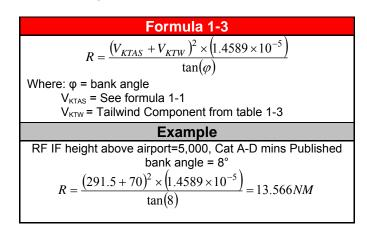
These criteria apply to construction at or below FL 190. Where turns above FL 190 are required, use a bank angle of 5°. If 5° results in a DTA value greater than 20 NM, then
