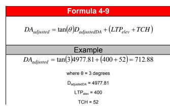
Finally, calculate the adjusted DA value using formula 4-9.
