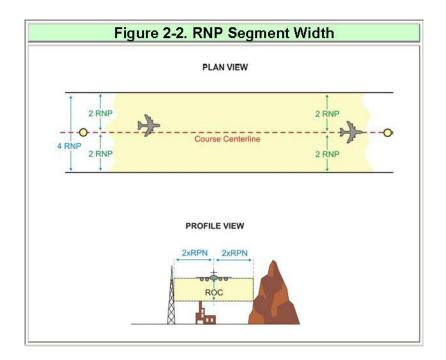
Apply the standard **RNP** values listed in table 2-1 unless a lower value is required to achieve the required ground track or lowest minimums. The lowest RNP values are listed in the "MINIMUM" column of table 2-1.
