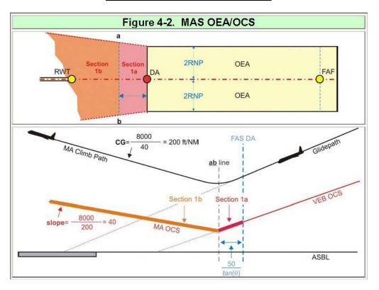
Calculate the MSL height of the missed approach surface (HMAS) at the **ab** line (**HMAS**<sub>ab</sub>) using formula 4-5.
