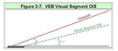
The OIS half-width at the LTP is 100 ft outside the runway edge. It splays at an angle of  $10^{\circ}$  relative to course until reaching a width of  $\pm$  1•RNP, which it maintains until contacting the final segment OEA at DA (see figure 3-8).
