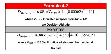
Where the 40:1 OCS is penetrated and the resulting HAT or visibility can be reduced by at least 50 ft or  $\frac{1}{4}$  SM respectively, consider limiting the MAS RNP value until clearing the obstruction. Use the largest RNP value (FAS RNP $\leq$ 1.0) that clears the obstruction. The maximum distance (NM) (**D**MASRNP) that the < 1.0 RNP value may be extended into the MAS is calculated using formula 4-3 (see figure 4-1B).
