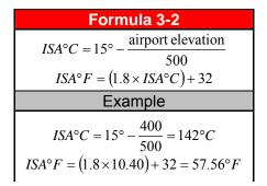
The approach procedure should offer obstacle protection within a temperature range that can reasonably be expected to exist at the airport. Establish the lower temperature limit from the 5-year average lowest temperature for the coldest month of the year (ACT). Determine the difference ( $\Delta$ ISALOW) between this temperature and ISA temperature for the airport using formula 3-3.
