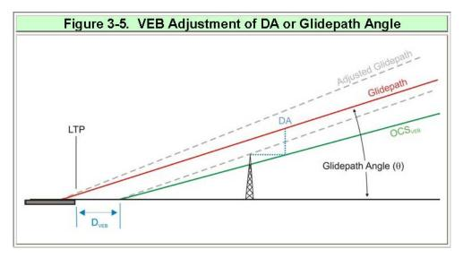
NOTE: DVEB decreases slightly when glidepath angle is increased. Therefore if the angle is increased to accommodate a penetration, the VEB must be recalculated and the OCS re-evaluated.
