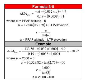
Determine the **published** low temperature limitation for the procedure derived from formula 3-6, using the  $\Delta$ **ISA**Low derived from formula 3-3 or 3-5 as appropriate. If the temperature history for the location indicates the low temperature limitation is frequently encountered during established busy recovery times, consider raising the glidepath angle to the lowest angle (within table 3-1 limits) that will make the approach usable more often.
