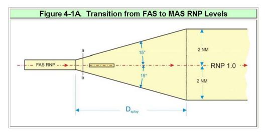
The along-track distance (NM) required to complete the splay may be calculated using formula 4-1.
