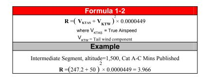
**1.11.2 a. Turn Radii Based On Nonstandard Bank Angles.** The standard design bank angle is 18°. Lower or higher bank angles are allowed for smooth transitions, maintaining stabilized approaches, lower minima, or achieve specific leg lengths (see formula 1-3). Nonstandard bank angles must fall in the window of values listed in table 1-4.
