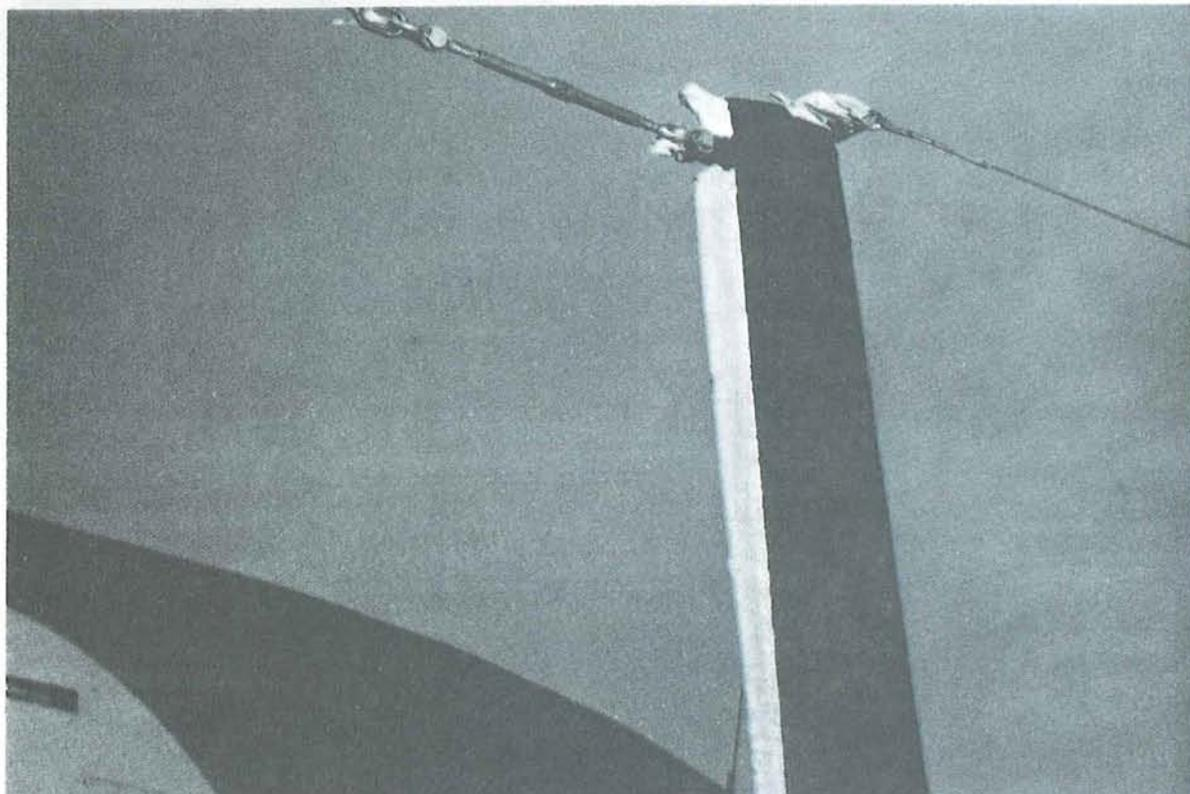
FIGURE 97. Clear ice on an aircraft antenna mast.
