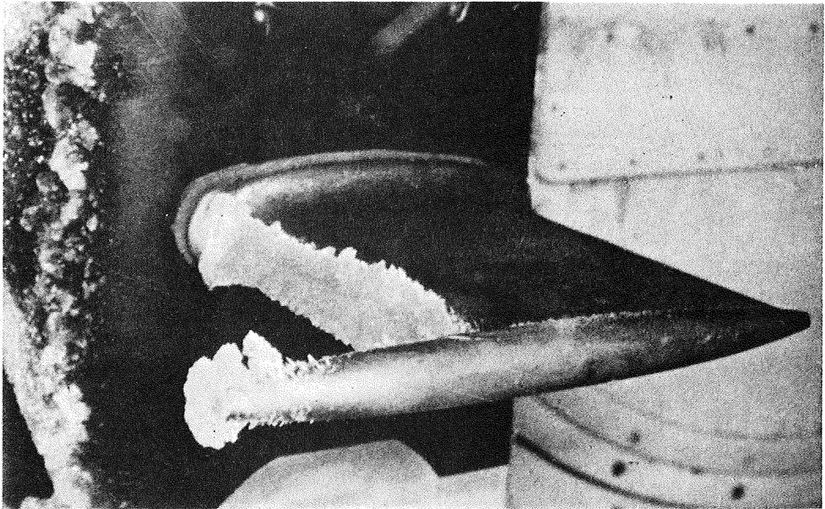
FIGURE 94. External icing on a pitot tube.
