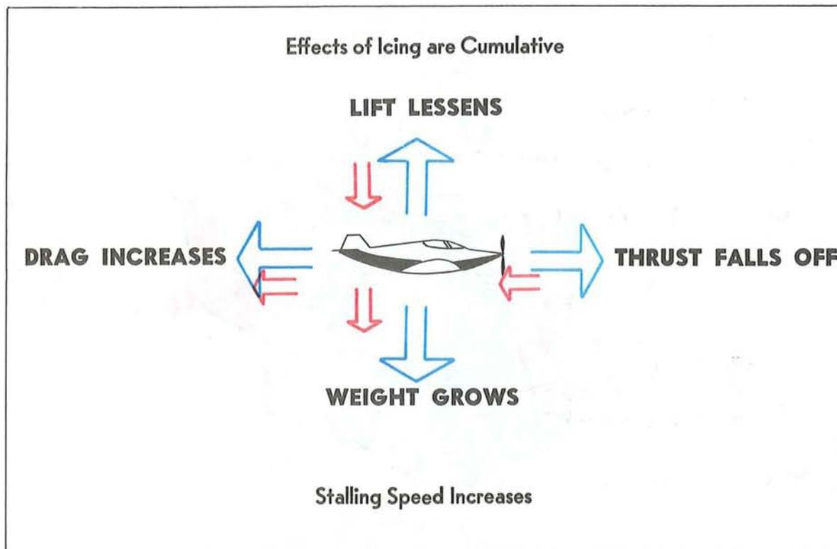
FIGURE 89. Effects of structural icing.
