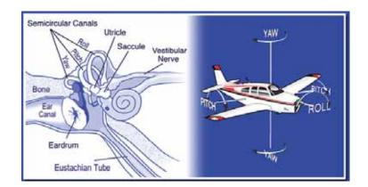
Each canal is filled with a fluid called endolymph and contains a motion sensor with little hairs whose ends are embedded in a gelatinous structure called the cupula. The cupula and the hairs move as the fluid moves inside the canal in response to an angular acceleration.
