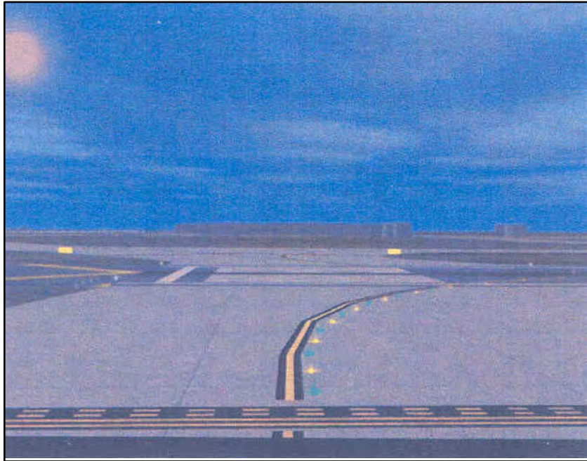
FIG 2-1-12 Taxiway Lead-On Light Configuration
