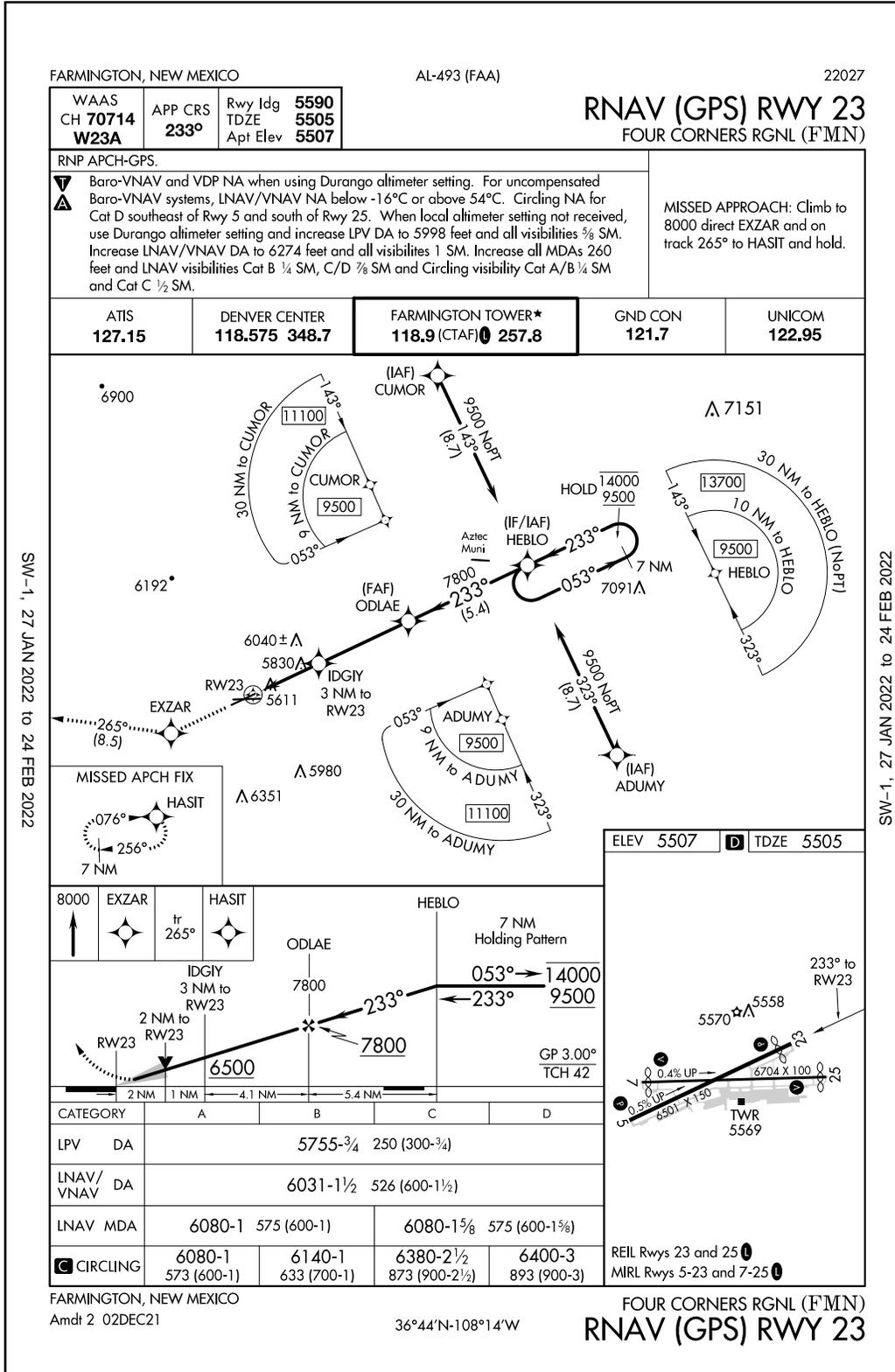
**12.4.7** TAAs may be modified from the standard size and shape to accommodate operational or ATC requirements. Some areas may be eliminated, while the other areas are expanded. The “T” design may be modified by the procedure designers where required by terrain or ATC considerations. For instance, the “T” design may appear more like a regularly or irregularly shaped “Y,” upside down “L,” or an “L.”
