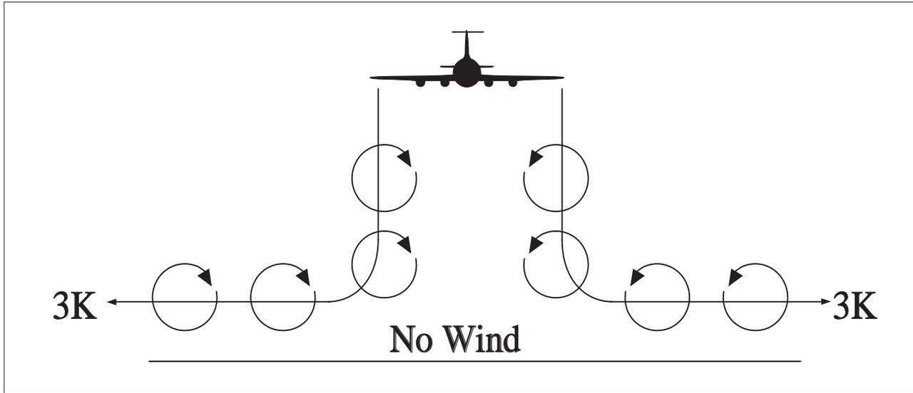
**28.4.1.4** When the vortices of larger aircraft sink close to the ground (within 100 to 200 feet), they tend to move laterally over the ground at a speed of 2 or 3 knots. (See FIG GEN 3.5-21.)
