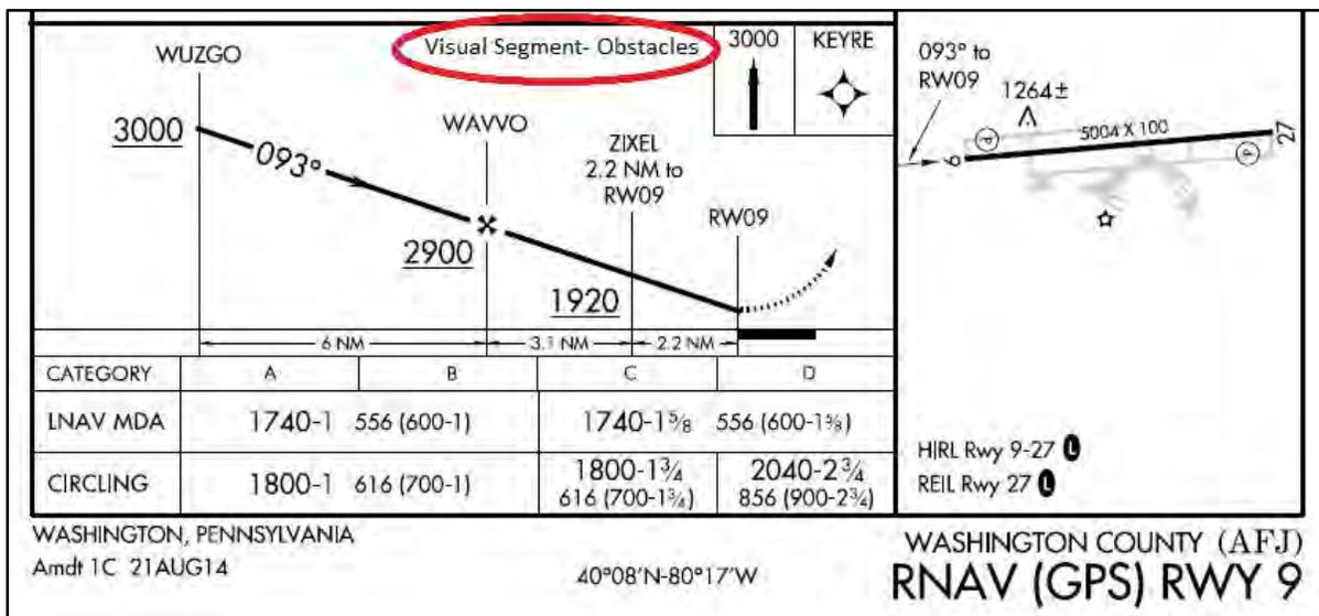
**12.11.3** Pilots may use the published angle and estimated/actual groundspeed to find a target rate of descent from the rate of descent table published in the back of the U.S. Terminal Procedures Publication. This rate of descent can be flown with the Vertical Velocity Indicator (VVI) in order to use the VDA as an aid to flying a stabilized descent. No special equipment is required.
