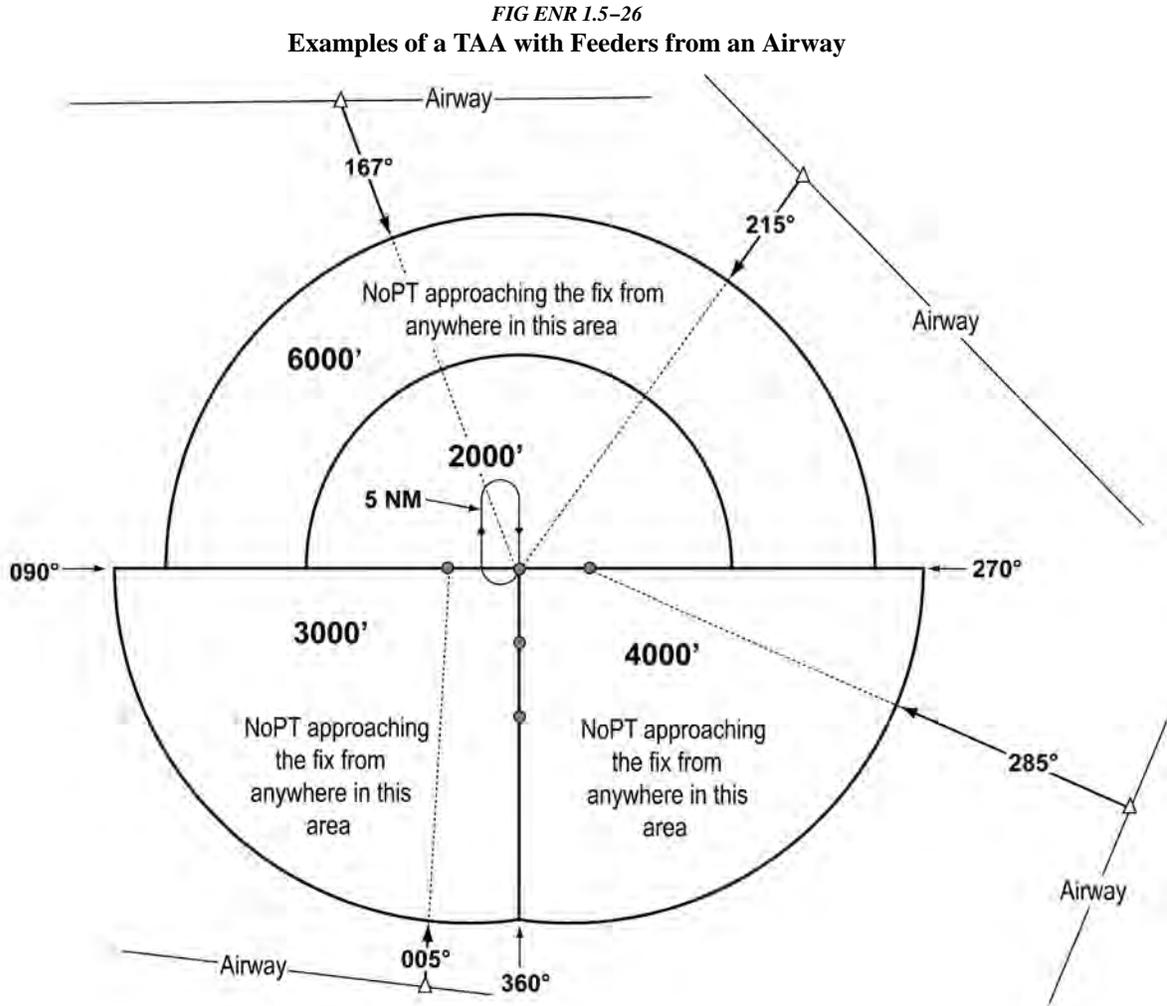
**12.4.9** Each waypoint on the “T” is assigned a pronounceable 5-letter name, except the missed approach waypoint. These names are used for ATC communications, RNAV databases, and aeronautical navigation products. The missed approach waypoint is assigned a pronounceable name when it is not located at the runway threshold.
