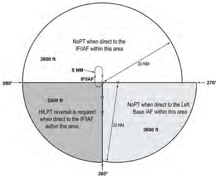
**12.4.8** When an airway does not cross the lateral TAA boundaries, a feeder route will be established from an airway fix or NAVAID to the TAA boundary to provide a transition from the en route structure to the appropriate IAF. Each feeder route will terminate at the TAA boundary and will be aligned along a path pointing to the associated IAF. Pilots should descend to the TAA altitude after crossing the TAA boundary and cleared for the approach by ATC. (See FIG ENR 1.5-26.)
