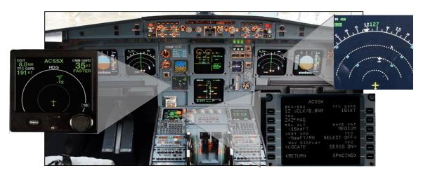
ADS-B is the underlying technology being utilized. The pilot performing the CAVS operation must have an ADS-B In system with CAVS capability with an appropriate Cockpit Display of Traffic Information (CDTI) and the traffic-to-follow (TTF) aircraft must have ADS-B Out capability. Virtually all aircraft operating at high-volume airports are ADS-B Out equipped. American Airlines is equipping its entire A321 fleet with ADS-B In equipment over the next 4-5 years.
