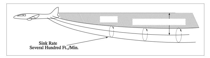
FIG 7-4-5 Vortex Movement Near Ground – No Wind
