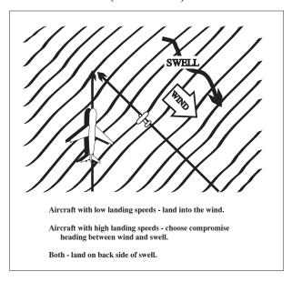
FIG 6-3-5 Wind-Swell-Ditch Heading
