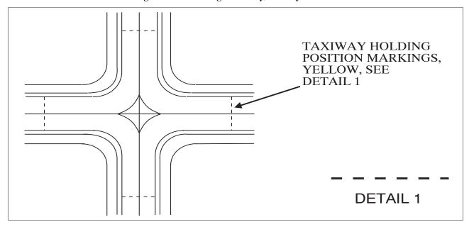
FIG 2-3-18 Vehicle Roadway Markings
