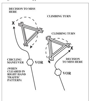
FIG 5-4-30 Circling and Missed Approach Obstruction Clearance Areas
