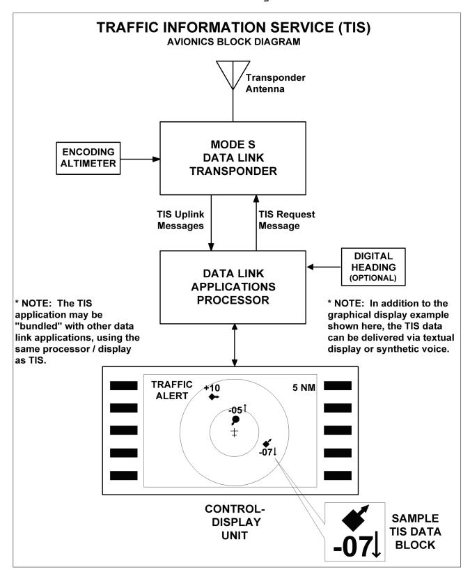
2. The cockpit equipment functionality required by a TIS client aircraft to receive the service consists of the following (refer to FIG 4-5-5):
