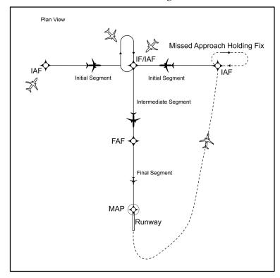
**3.** The standard TAA based on the "T" design consists of three areas defined by the Initial Approach Fix (IAF) legs and the intermediate segment course beginning at the IF/IAF. These areas are called the straight–in,
