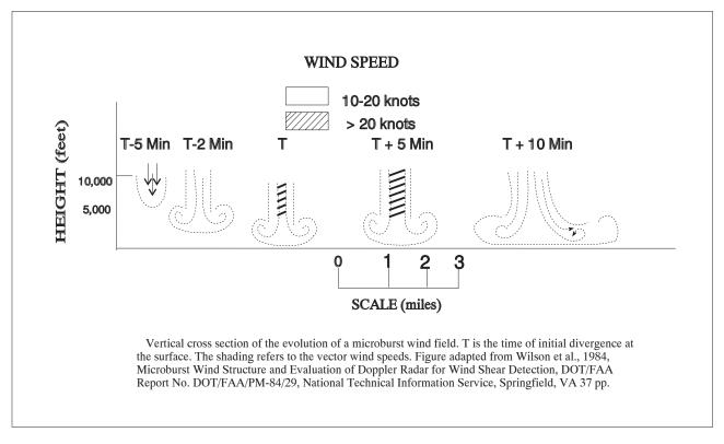
**c.** The life cycle of a microburst as it descends in a convective rain shaft is seen in FIG 7–1–13. An important consideration for pilots is the fact that the microburst intensifies for about 5 minutes after it strikes the ground.
