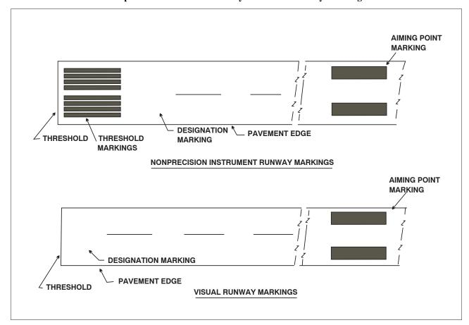
FIG 2-3-2 Nonprecision Instrument Runway and Visual Runway Markings
