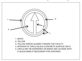
FIG 2-3-21 Nonmovement Area Boundary Markings
