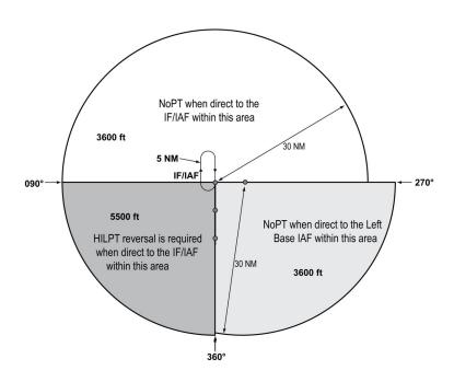
**8.** When an airway does not cross the lateral TAA boundaries, a feeder route will be established from an airway fix or NAVAID to the TAA boundary to provide a transition from the en route structure to the appropriate IAF. Each feeder route will terminate at the TAA boundary and will be aligned along a path pointing to the associated IAF. Pilots should descend to the TAA altitude after crossing the TAA boundary and cleared for the approach by ATC. (See FIG 5–4–10).
