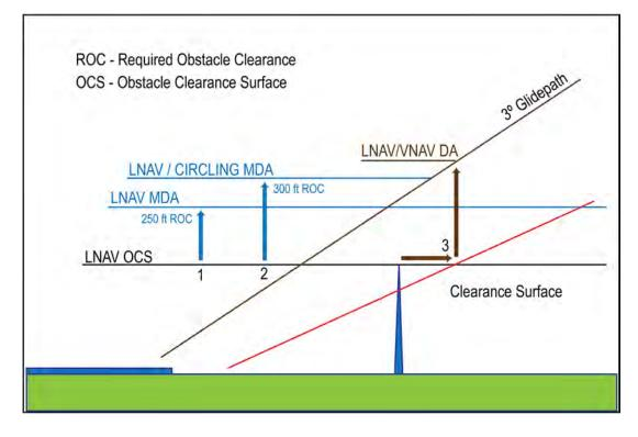
**12.7** FIG ENR 1.5–29 provides a visual representation of an obstacle evaluation and calculation of LNAV MDA, Circling MDA, LNAV/VNAV DA.
