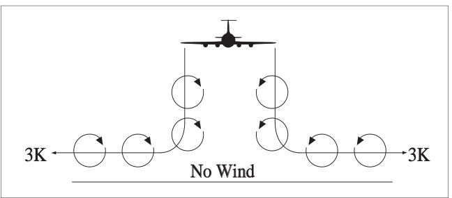
**28.4.1.4** When the vortices of larger aircraft sink close to the ground (within 100 to 200 feet), they tend to move laterally over the ground at a speed of 2 or 3 knots. (See FIG GEN 3.5–21.)
