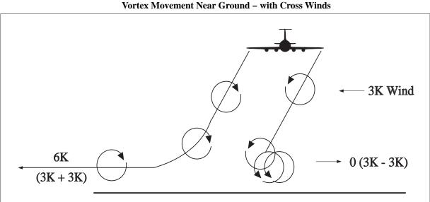
FIG GEN 3.5–22 Yortex Movement Near Ground – with Cross Winds
