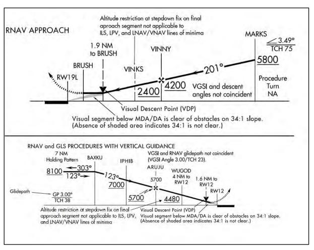
FIG ENR 1.5–17 Instrument Approach Procedure Stepdown Fixes
