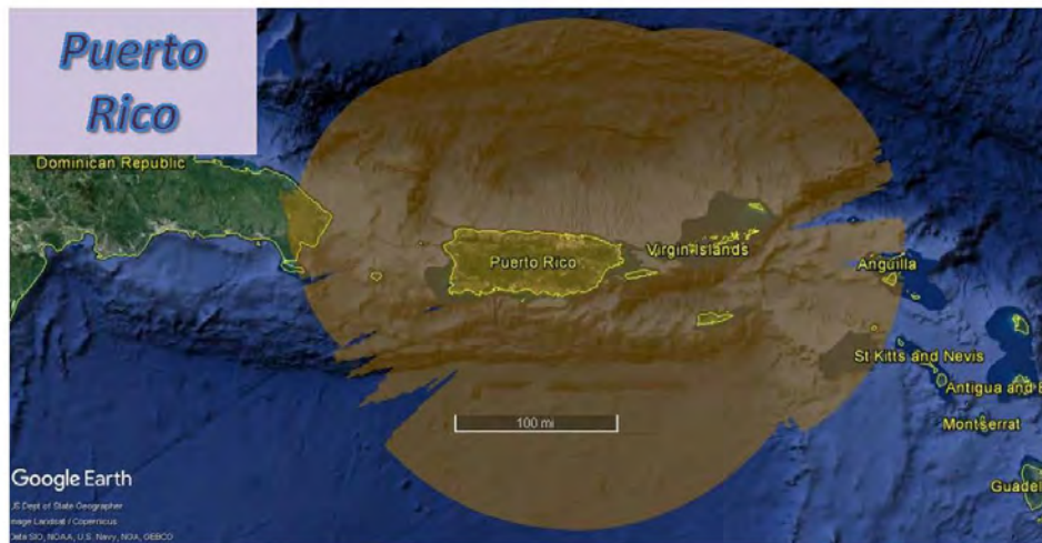
FIG ENR 1.6-II Hawaii, Puerto Rico, and Guam with ADS-B Coverage at 5,000' AGL
