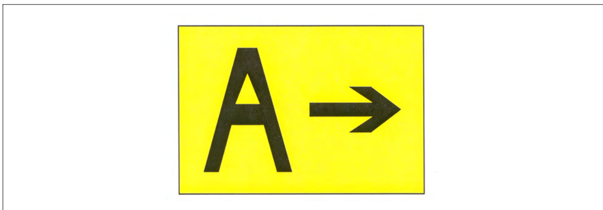
FIG AD 1.1-48 Direction Sign for Runway Exit
