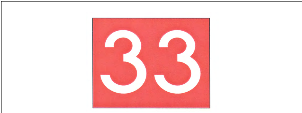
FIG AD 1.1-37 Holding Position Sign at Beginning of Takeoff Runway
