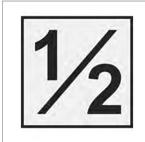
FIG ENR 5.7-1 Typical Runway Half-way Sign
