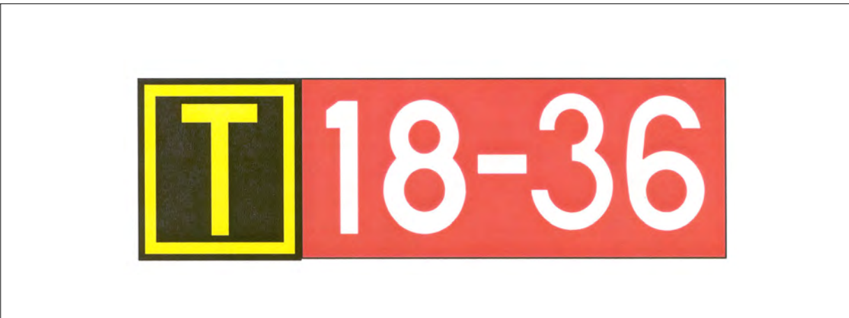
FIG AD 1.1-43 Taxiway Location Sign Collocated with Runway Holding Position Sign
