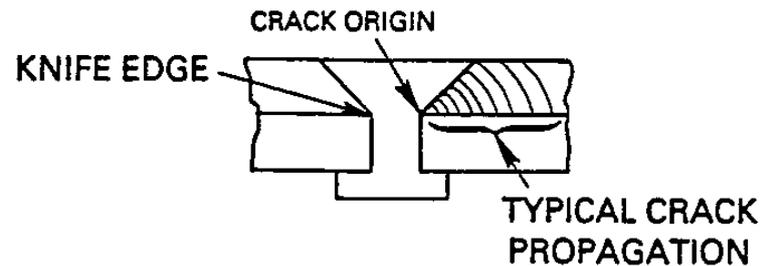
Figure 6b.--Cross section of a rivet and skin
