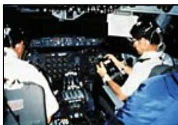
*NASA Cockpit Rest Study depicts pilots wired up with EEG and wrist activity monitoring equipment. The pilot on the right is completing a reaction time test with an early version of the psychomotor vigilance test.*
