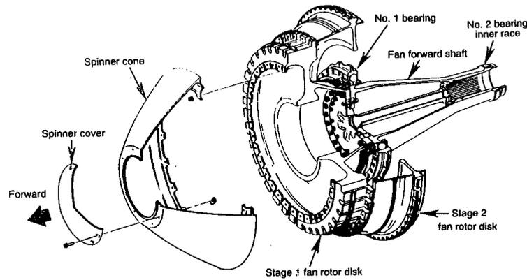
Figure 5.--CF6-6 fan rotor assembly.
