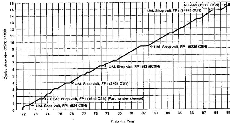
**Figure 9.--Inspection history of accident fan disk. (Data source GEAE)**
