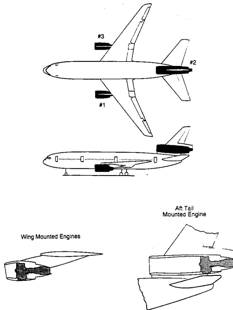
**Figure 1.--DC-10 airplane view illustrated with engine arrangement.**
