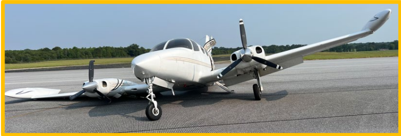
CE402 - Gear Collapse (AND) May 2025
