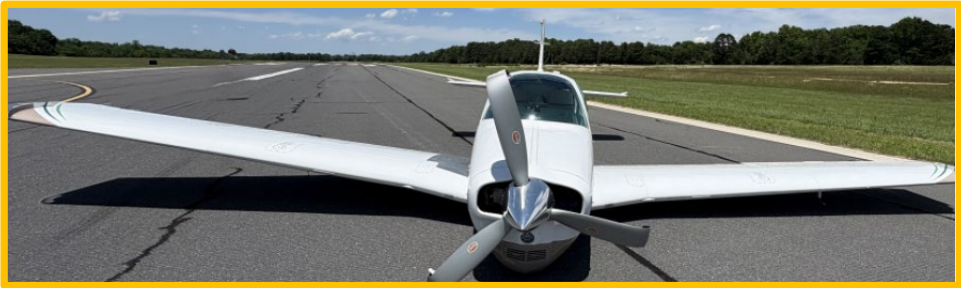
BE F33A - Failure to Extend Gear UZA – Rock Hill May 2025
