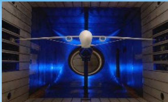
Transonic Truss-Braced Wing 5-10% fuel burn benefit
