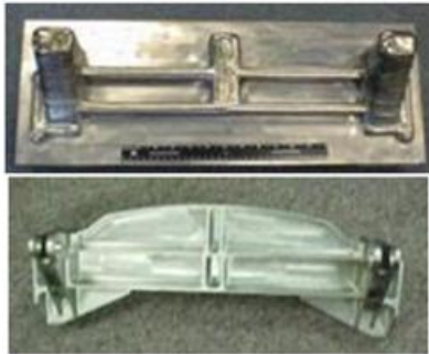
Speed brake Hinge Deposited on 36" x 8" x 2.5" Plate First Flying LAM Part
