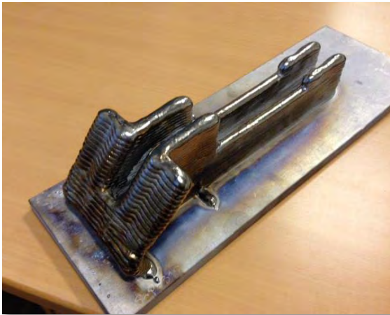
1st FAA-approved Titanium Structural Production Part - 787 Passenger Floor Support (shown in as-deposited condition)
