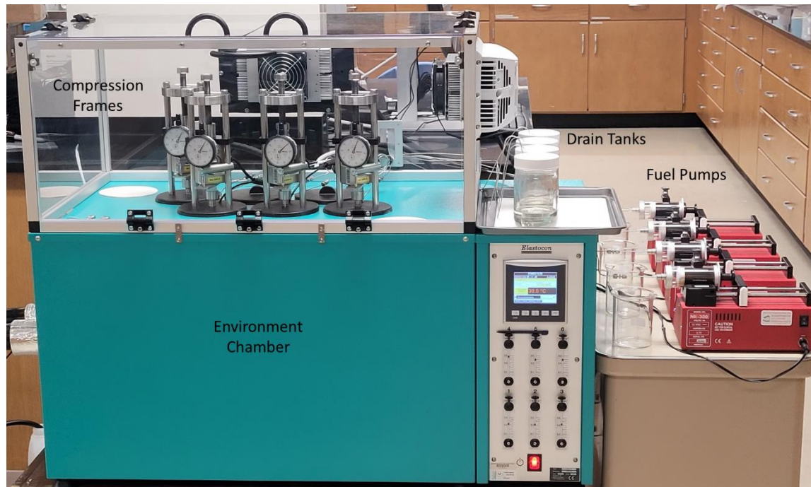
Figure 40. The assembled compressive stress relaxometer.
