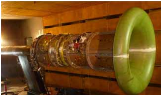
Figure 5-1. Integrated UHB Rig Installed in NASA Low-Speed Wind Tunnel Ready for Initial Break-In
