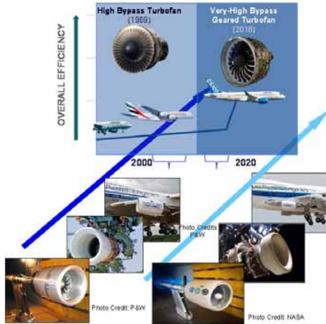
Figure 2-5. Fan Rig, Ground Engine, and Flight Tests Conducted in Late 2000s To Support 2016 GTF Entry Into Service; Same Process for UHB Technology, With Flight Testing To Be Conducted
