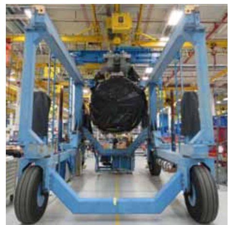
Figure 5-3. CLEEN UHB Engine (XGTF101-01) Being Installed on Shipping Stand for Delivery to West Palm Beach
