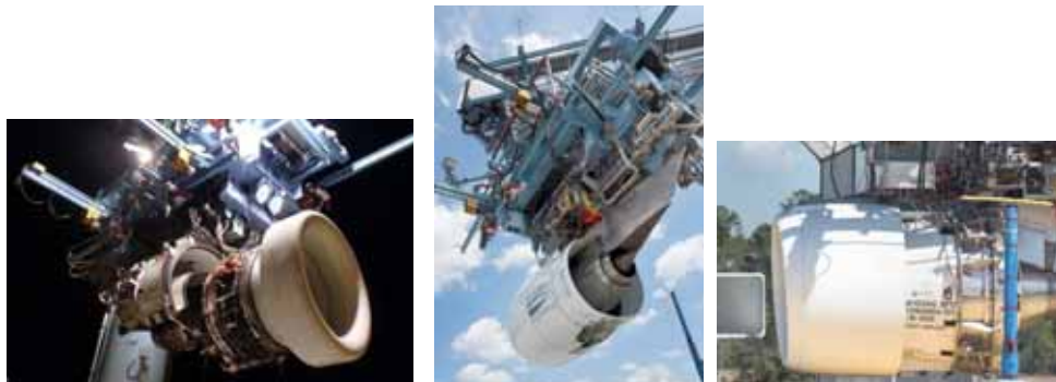
Figure 6-3. CLEEN UHB Engine (XGTF101-01) in Performance and Fan Mapping Configurations Installed in CII Test Stand (Fan Structural Response and Inlet Performance Testing Also Conducted in Configuration on Right)
