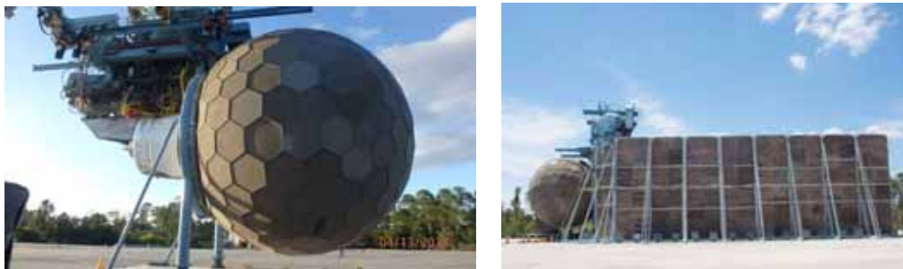
Figure 6-4. Illustration of Engine Configured With Inlet Control Device (Left) Used for Acoustic Testing and With Barrier Wall Installed for Forward/Aft Separation
