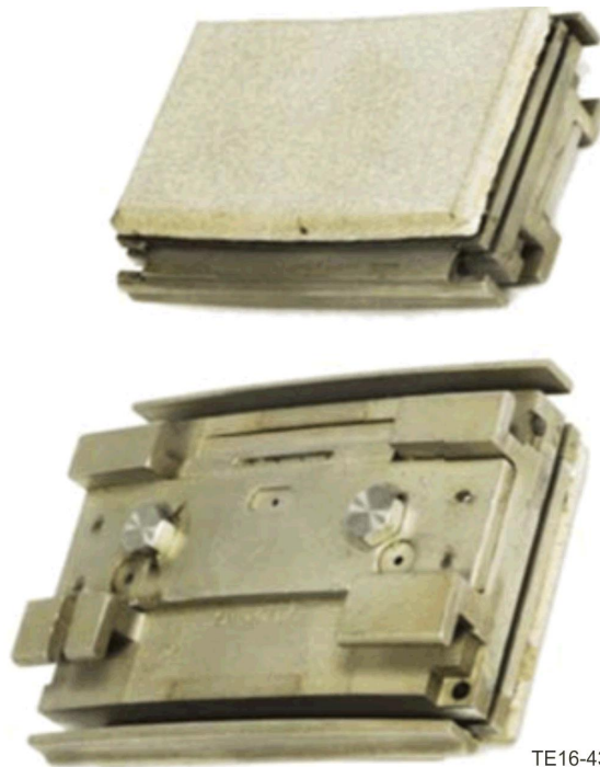
Figure 9. Representative blade track assembly.
