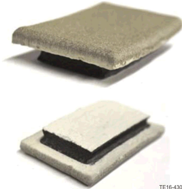
Figure 8. Representative coated (EBC and abrasion-resistant) SiC/SiC CMC hardware.
