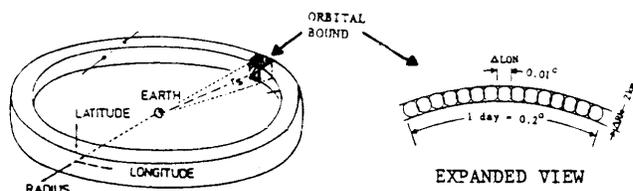
FIGURE 6-5. GEOSTATIONARY RING SHOWING SATELLITE ORBITAL BOUNDS
