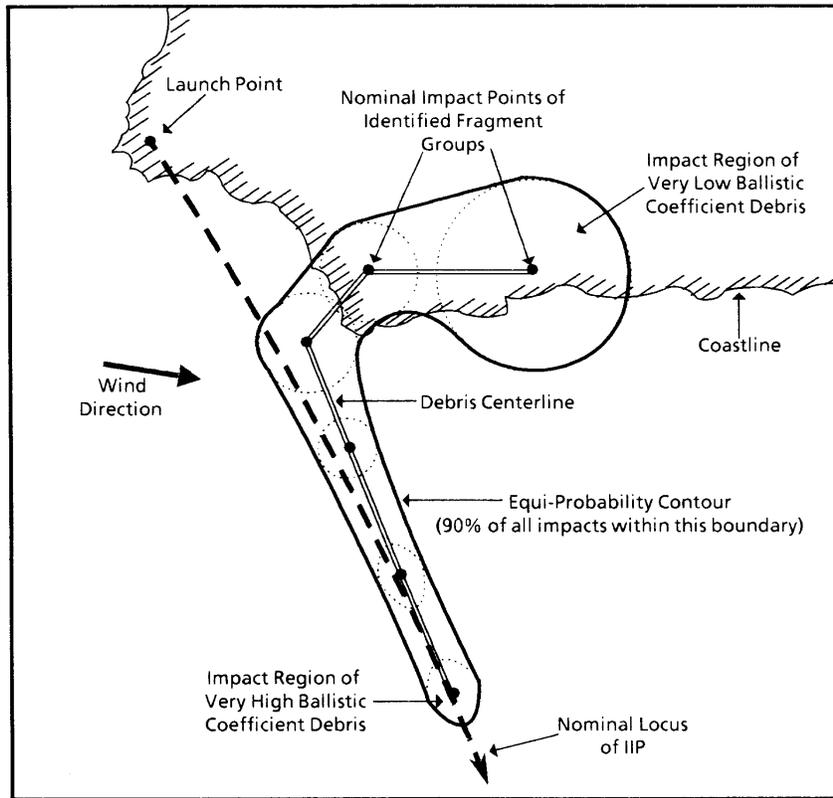
FIGURE 10-3. A TYPICAL DEBRIS DISPERSION AT IMPACT PATTERN
