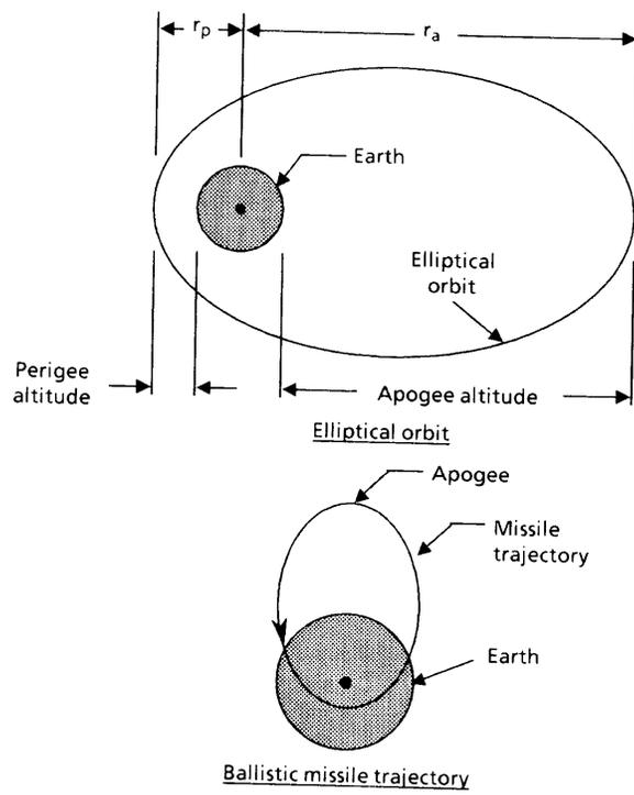
FIGURE 4-6. GEOMETRY OF SATELLITE ORBITS AND ELV TRAJECTORIES
