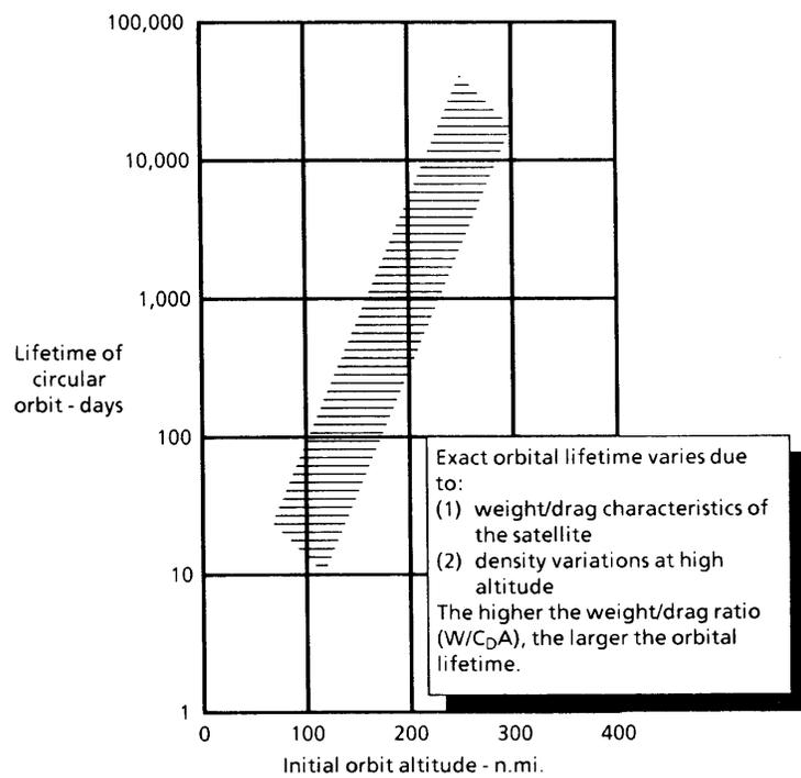
**FIGURE 4-3. APPROXIMATE LIFETIMES FOR SATELLITES IN CIRCULAR ORBITS**
