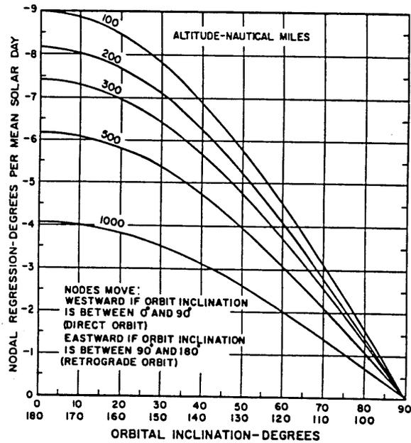
FIGURE 4-12. ORBITAL PLANE PRECESSION DUE TO EARTH'S OBLATENESS (Ref. 2)
