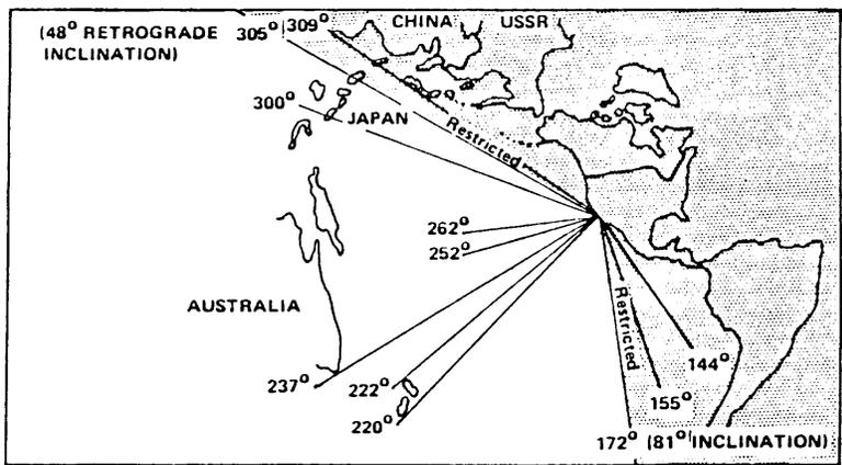
FIGURE 10-8. WTR GEOGRAPHIC LAUNCH AZIMUTH CONSTRAINTS (REF. 7)
