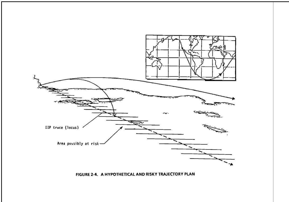
risk analyses are performed using models that consider the probability of the vehicle failing in a variety of modes and simulate the behavior of the missile during and after malfunction, including the effect of activating the flight termination system.
