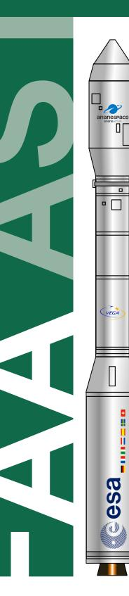
The Vega launch vehicle, named after the second brightest star in the northern hemisphere, is operated by Arianespace and targets payloads to polar and low Earth orbits used by scientific and Earth observation satellites. It is manufactured by ELV SpA, a joint venture between Italybased Avio SpA and the Italian Space Agency (ISA).
