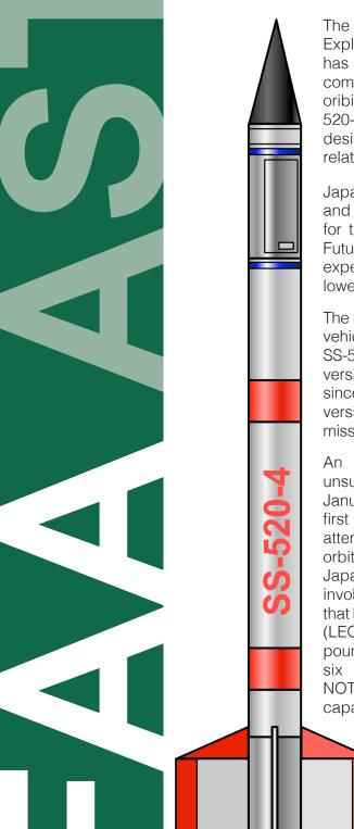
The Japan Aerospace and Exploration Agency (JAXA) has been working with several companies to develop a very small oribital launch vehicle. The SS-520-5 is a development vehicle designed to gather data for use in related future programs.
