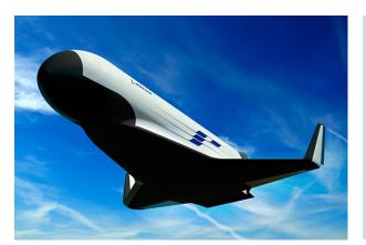
Boeing is the lead on the development of this team's XS-1 concept. Boeing is leveraging its extensive spaceflight experience, perhaps with emphasis on its X-37B spaceplane, which is owned and operated by the U.S. Air Force. Its concept is to deploy the XS-1 via an aircraft. The spaceplane would then deploy the payload and return to Earth as an airplane. Blue Origin is focusing on the propulsion system. (Source: Boeing)
