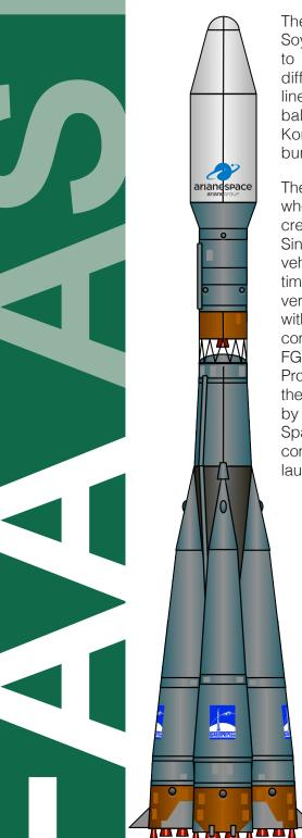
The Soyuz 2 (also referred to as Soyuz ST) is used to launch satellites to virtually any orbit from three different launch sites. It can trace its lineage to the R-7 intercontinental ballistic missile designed by Sergei Korolov and his OKB-1 design bureau in the mid-1950s.
