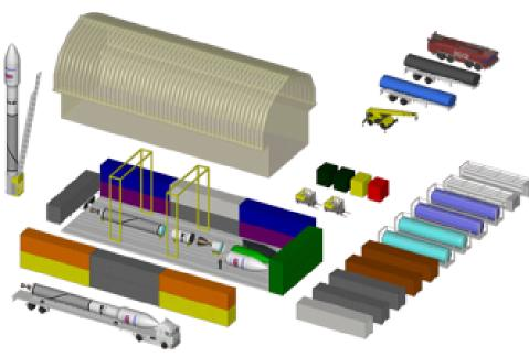
The Black Arrow 2 launch facility is unique in that it is designed to be transported to various launch sites depending on customer needs. All the facilities can be stowed in 26 standard ISO cargo-containers and can be relocated to a new launch site in less than 30 days. (Source: Horizon Space Technologies)
