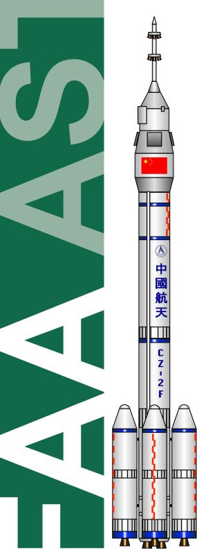
The Long March 2F, introduced in 1999, is China's only vehicle designed to transport astronauts. The two-stage vehicle is ultimately derived from the Long March 2C via the Long March 2E, a retired vehicle that was used to send payloads to geosynchronous orbit (GEO).
