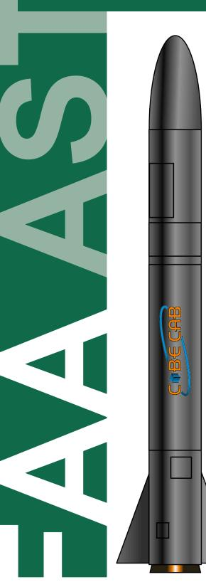
U.S.-based CubeCab is а company seeking to provide dedicated launches for operators of CubeSats. The relatively small vehicle will be launched from an F-104 Starfighter offered by Starfighters Aerospace that will take off from NASA's Shuttle Facility at Kennedy Landing Space Center (KSC) in Florida. The CubeCab vehicle will be attached below the wing of the F-104 in a similar manner to an air-to-air missile.
