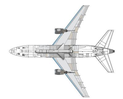
Orbital ATK uses a modified L-1011 aircraft to carry and launch the Pegasus XL vehicle. The ground equipment necessary to launch the system is minimal, and the combination can be launched from almost any conventional runway.
