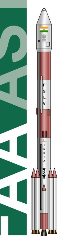
The Indian Space Research Organization (ISRO) has offered the Polar Satellite Launch Vehicle (PSLV) since 1993. The vehicle is used to launch small and medium payloads to low Earth orbit and, on occasion, to send small satellites to geosynchronous orbit. For missions to LEO, it is not uncommon for the PSLV to launch several satellites at a time.
