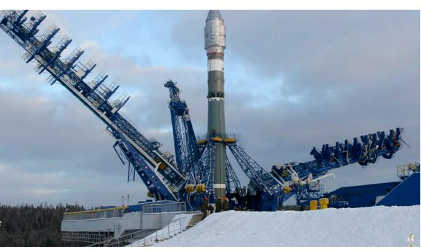
A Soyuz 2.1v is prepared for launch in December 2015. The launch, carrying a Kanopus remote sensing satellite, did not go entirely as planned - the payload did not fully separate from the upper stage due to a second stage latching problem. (Source: Russian MoD)
