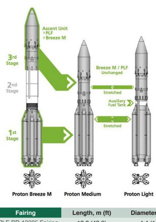
An ILS graphic showing the differences between the Proton M, the Proton Medium, and the Proton Light. The latter version is apparently no longer being developed. (Source: ILS)
