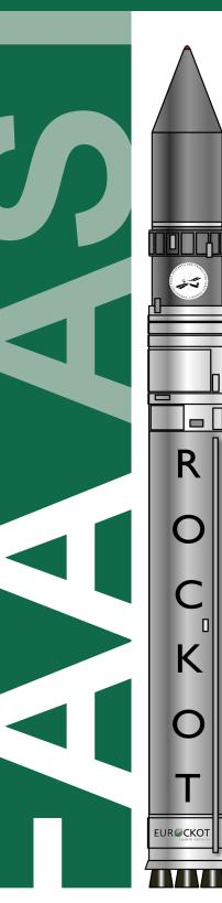
The three-stage Rockot is developed using refurbished missile components. The missile used as the basis for the commercially available vehicle is the UR100N (SS-19) intercontinental ballistic missile (ICBM) built by Soviet-era OKB-52. Production and launch of the Rockot is managed by Eurockot Launch Services GmbH, a joint company between Russia's Khrunichev State Research and Production Space Center and EADS Astrium.
