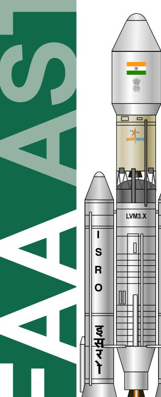
The LVM3, formally called the Geosynchronous Space Launch Vehicle Mark III (GSLV Mk III), is a launch vehicle being developed by the Indian Space Researc organization (ISRO). It is designed to enable India to achieve complete self reliance in terms of sending satellites to geosynchronous orbits (GEO). Currently, India largely depends on Europe's Ariane 5 ECA to send ISRO payloads to GEO.
