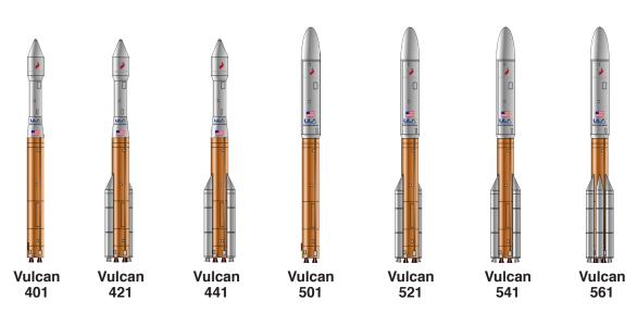
The Vulcan will feature a core stage and a combination of up to six solid rocket boosters, two Centaur upper stage options (and later ACES), and a 4- or 5-meter fairing. There will be three versions of the 400 series and four versions of the 500 series.
