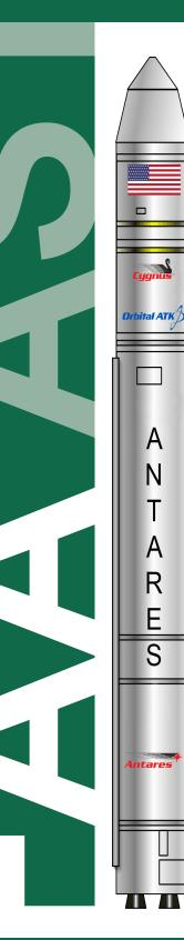
In 2013, Orbital Sciences Corporation (now Orbital ATK) began offering its Antares, a two-stage vehicle designed to launch government and commercial satellites to low Earth orbit (LEO), Cygnus cargo modules to the International Space Station (ISS), and missions requiring Earth escape trajectories. The Antares is also available under the NASA Launch Services (NLS) II contract for future science missions.
