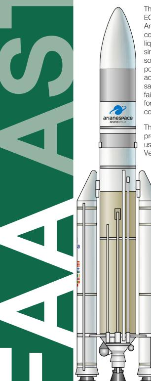
The Ariane 5, technically the Ariane 5 ECA, is the workhorse of France-based Arianespace, a European launch consortium. The Ariane 5 consists of a liquid-fueled core stage powered by a single Vulcain 2 engine, two strap-on solid boosters, a cryogenic upper stage powered by an HM7B engine, a payload adapter that can accommodate two satellites (called SYLDA), and a payload fairing. The Ariane 5 ECA is optimized for launches of two geosynchronous communications satellites.
