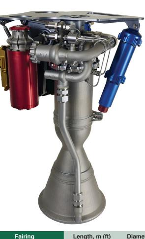
Rocket Lab's Rutherford engine. All its primary components are produced using additive manufacturing, or 3D printing. (Source: Rocket Lab)
