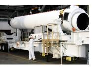
A GEM-60 being prepared for integration on a Delta IV (Orbital ATK)
