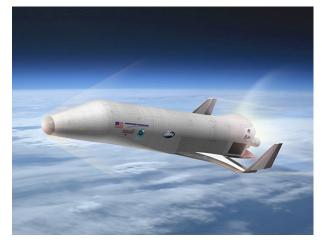
Northrop Grumman's subsidiary, Scaled Composites, is developing this team's XS-1 concept. The concept includes a clean-pad approach using a transporter erector launcher with minimal infrastructure and ground crews, highly autonomous flight operations, and horizontal landing and recovery on standard runways. Virgin Galactic would manage operational missions. (Source: Northrop Grumman)
