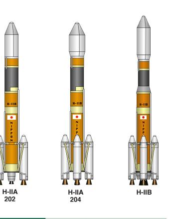
The H-IIA is used for a variety of missions and represents the workhorse launch vehicle for Japan. The H-IIB has been used exlusively to send cargo to the ISS, but recently MHI Launch Services has made the vehicle avalabile for commercial use.
