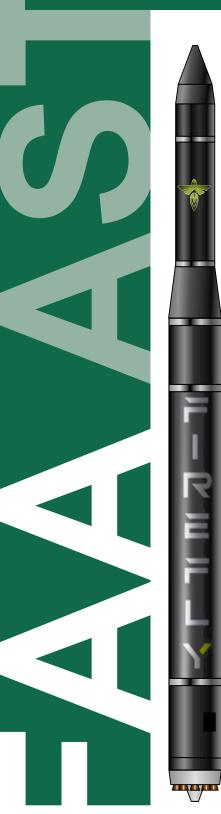
U.S.-based company Firefly Aerospace Inc. ("Firefly") plans to offer the Alpha launch vehicle to service the burgeoning smallsatellite industry. Alpha is a two-stage vehicle, utilizing composite materials to create strong lightweight primary structures such as the airframe and propellant tanks.
