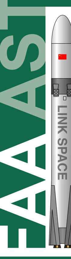
China-based Link Space, founded in 2014, is developing a two-stage, small orbital launch vehicle called New Line 1 (Xin Gan Xian 1) with a reusable first stage. The vehicle is based on a successfully tested suborbital rocket called KC-SA-TOP.
