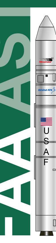
The Minotaur IV is an orbital launch vehicle offered by Orbital ATK. The vehicle is derived from the Peacekeeper intercontinental ballistic missile (ICBM).
