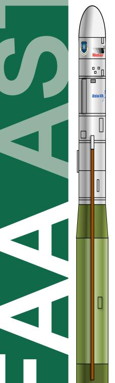
Orbital ATK provides the Minotaur I as a responsive and cost-effective launch solution for U.S. Government spacecraft. The launch vehicle is composed of residual 1960s era Minuteman II first and second stage solid rocket motors integrated with Orion upper stages.
