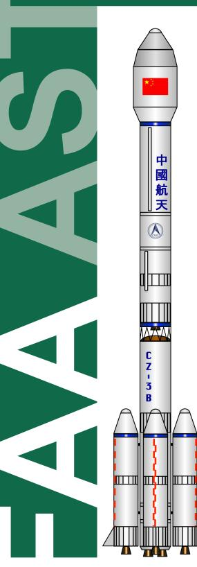
With a low Earth orbit (LEO) capacity of 12,000 kg (26,456 lb), the Long March 3B is currently China's most powerful launch vehicle. The vehicle is derived from the Long March 3A vehicle, with the key difference being that the Long March 3B uses four liquid boosters. The vehicle is primarily used for missions to a geostationary transfer orbit (GTO), but can be used for uncrewed science missions to the Moon (Chang'e-3).
