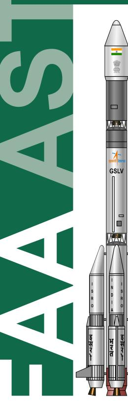
The Geosynchronous Satellite Launch Vehicle (GSLV) project began in 1990 with the objective of achieving an indigenous satellite launch capability to geosynchronous orbit (GEO). The vehicle was developed by the Indian Space Research organization (ISRO).
