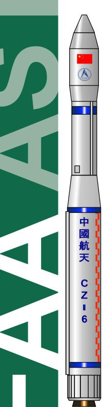
The Long March 6 is a cooperative effort between China Aerospace Science and Technology Corporation (SAST) and the China Academy of Launch Vehicle Technology (CALT). It is a small, liquidfueled vehicle that has a low Earth orbit (LEO) payload capacity less than that provided by the currently available small-class Long March 2C, meaning the vehicle serves a niche previously not directly addressed.
