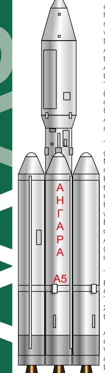
The Khrunichev State Research and Production Space Center has been developing the Angara series of vehicles to replace virtually all vehicles in service with the exception of the Soyuz. The Angara 1.2 is expected to replace the Rockot and Dnepr while the Angara A5 is expected to replace the Proton M within 5-7 years. The Universal Rocket Module (URM-1) forms the modular core of every Angara vehicle, with a URM-2 used as a second stage. A Breeze-M upper stage serves as an optional third stage.
