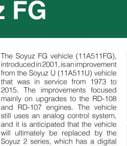
The vehicle is used for crewed Soyuz missions to the International Space Station (ISS). It is also used to deliver the Progress cargo modules to ISS. The Soyuz FG can also be outfitted with a Fregat upper stage for certain missions; examples of missions using Fregat include Mars Express and some replenishments of the Globalstar constellation. Launch Service Provider VKS/Glavkosmos
