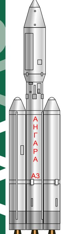
The Khrunichev State Research and Production Space Center has been developing the Angara series of vehicles to replace virtually all vehicles in service with the exception of the Soyuz. The Angara 1.2 is expected to replace the Rockot and Dnepr while the Angara A5 is expected to replace the Proton M. The Universal Rocket Module (URM-1) forms the modular core of every Angara vehicle, with a URM-2 used as a second stage. A Breeze-M upper stage serves as an optional third stage.
