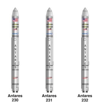
The Antares is offered in three variants. The first stage, which is common to all variants, is outfitted with a CASTOR 30XL solid motor upper stage. The vehicle can have no third stage, or an option between a Bi-Propellant Third Stage (BTS) or a STAR 48. The same fairing is used for all six versions.
