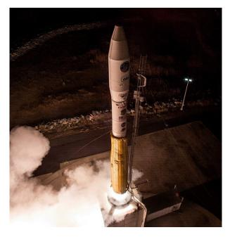
A Minotaur I lifts off from MARS on November 20, 2013 carrying 29 payloads. At the time, this was a U.S. record for number of payloads launched at once. Note the insulative blanket, which peels away seconds after lift off. (Source: Orbital ATK)
