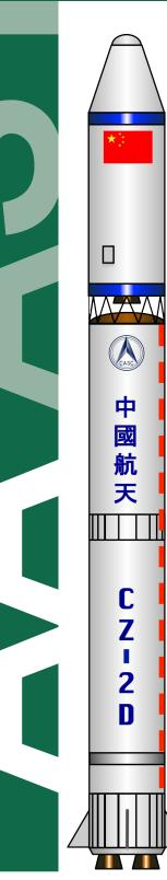
Primarily used to lift payloads to LEO and SSO, the 41-meter-tall, two-stage Long March 2D launch vehicle is part of the Long March 2 family of rockets. First launched from Jiuquan Satellite Launch Center in 1992, this Chinese launch vehicle has completed 25 successful launches. Two variants of the Long March 2D are known, and both are two-stage rockets that employ engines fueled by  $N_2O_4/UDMH$ .
