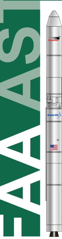
The Minotaur VI, offered by Orbital ATK, is derived from the Minotaur IV+. The five-stage vehicle is essentially identical to the Minotaur IV, except that it features an additional SR-118 solid motor stage. The only new piece of hardware is the interstage assembly that separates the two SR-118 stages.
