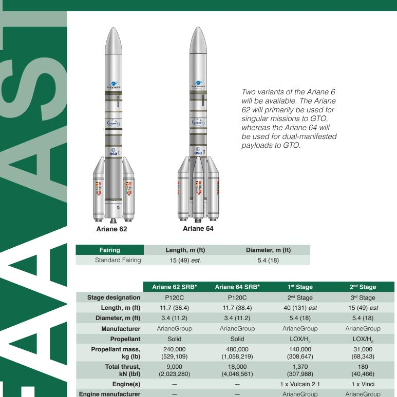
\* Figures are for each booster. Propellant mass and total thrust is sum of all boosters.
