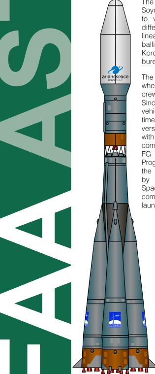
The Soyuz 2 (also referred to as Soyuz ST) is used to launch satellites to virtually any orbit from three different launch sites. It can trace its lineage to the R-7 intercontinental ballistic missile designed by Sergei Korolov and his OKB-1 design bureau in the mid-1950s.
