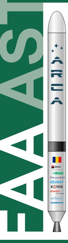
Developed by the Aeronautics and Cosmonautics Romanian Association (ARCA) as part of its bid to win the Google Lunar X Prize, the Haas 2C is a 2-stage orbital launch vehicle. The vehicle is named after Transylvanian Conrad Haas, an engineer that explored staged rockets during the 16th century, well before Konstantin Tsiolkovsky published his rocket equation in 1903. In addition to rocket technology, ARCA develops aeronautical and ground transportation systems.
