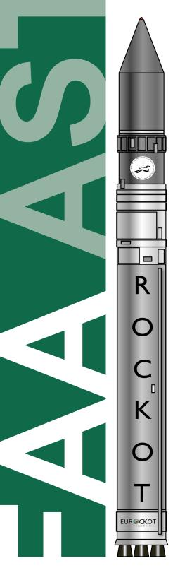
The three-stage Rockot is developed using refurbished missile components. The missile used as the basis for the commercially available vehicle is the UR100N (SS-19) intercontinental ballistic missile (ICBM) built by Soviet-era OKB-52. Production and launch of the Rockot is managed by Eurockot Launch Services GmbH, a joint company between Russia's Khrunichev State Research and Production Space Center and EADS Astrium.
