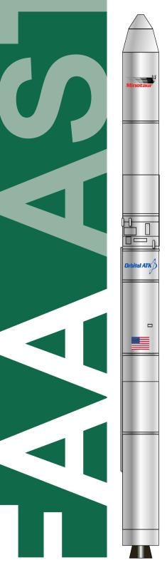
The Minotaur VI, offered by Orbital ATK, is derived from the Minotaur IV+. The five-stage vehicle is essentially identical to the Minotaur IV, except that it features an additional SR-118 solid motor stage. The only new piece of hardware is the interstage assembly that separates the two SR-118 stages.
