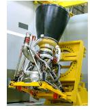
An RS-68A being prepared for installation on a Delta IV CBC (Aerojet Rocketdyne)
