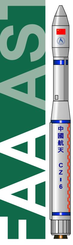
The Long March 6 is a cooperative effort between China Aerospace Science and Technology Corporation (SAST) and the China Academy of Launch Vehicle Technology (CALT). It is a small, liquid-fueled vehicle that has a low Earth orbit (LEO) payload capacity less than that provided by the currently available small-class Long March 2C, meaning the vehicle serves a niche previously not directly addressed.
