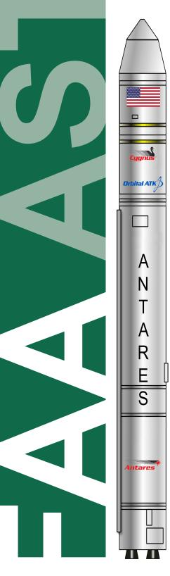
In 2013, Orbital Sciences Corporation (now Orbital ATK) began offering its Antares, a two-stage vehicle designed to launch government and commercial satellites to low Earth orbit (LEO), Cygnus cargo modules to the International Space Station (ISS), and missions requiring Earth escape trajectories. The Antares is also available under the NASA Launch Services (NLS) II contract for future science missions.
