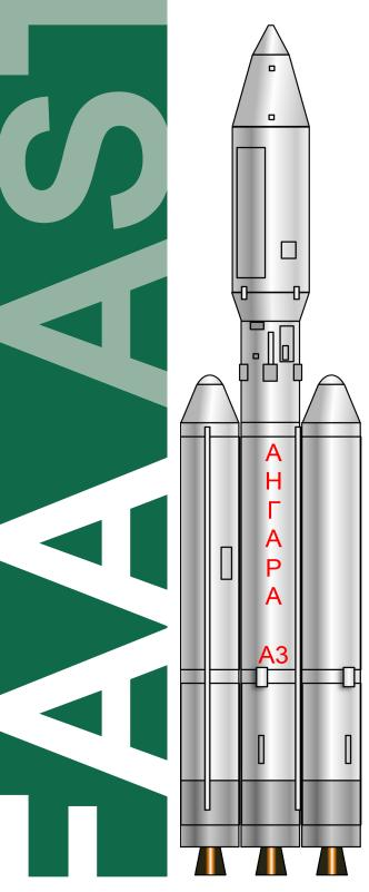
The Khrunichev State Research and Production Space Center has been developing the Angara series of vehicles to replace virtually all vehicles in service with the exception of the Soyuz. The Angara 1.2 is expected to replace the Rockot and Dnepr while the Angara A5 is expected to replace the Proton M. The Universal Rocket Module (URM-1) forms the modular core of every Angara vehicle, with a URM-2 used as a second stage. A Breeze-M upper stage serves as an optional third stage.
