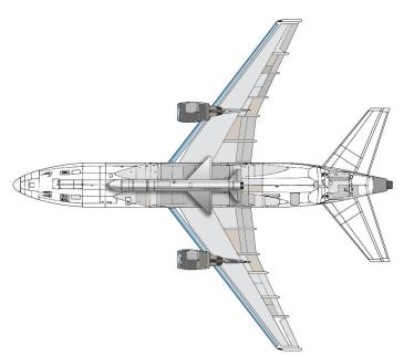
Orbital ATK uses a modified L-1011 aircraft to carry and launch the Pegasus XL vehicle. The ground equipment necessary to launch the system is minimal, and the combination can be launched from almost any conventional runway.
