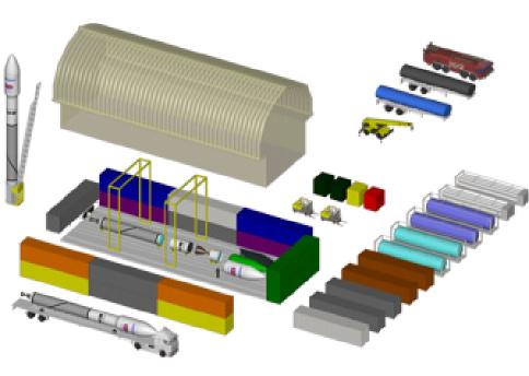
The Black Arrow 2 launch facility is unique in that it is designed to be transported to various launch sites depending on customer needs. All the facilities can be stowed in 26 standard ISO cargo-containers and can be relocated to a new launch site in less than 30 days. (Source: Horizon Space Technologies)
