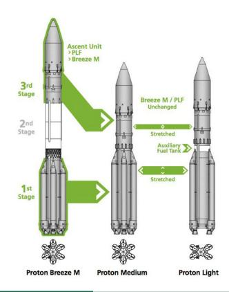
An ILS graphic showing the differences between the Proton M, the Proton Medium, and the Proton Light. The latter version is apparently no longer being developed. (Source: ILS)
