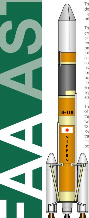
The two-stage H-IIA and H-IIB, designed and built by Mitsubishi Heavy Industries (MHI), are Japan's primary launch vehicles.
