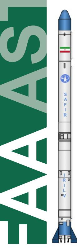
Iran's Safir launch vehicle is based on the Shahab 3 ballistic missile. The Shahab 3. based on the North Korean Nodong-1 ballistic missile, was in service from 1998 through 2003. Though the Safir may have been launched during an attempt in 2007 (there is confusion on what vehicle was used during the flight test), the first confirmed launch of Safir occured in 2008. This suborbital flight was followed by six orbital launch attempts, four of which have been considered successful.
