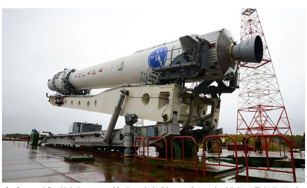
An Angara 1.2 vehicle is prepared for launch, in this case for a suborbital test flight that took place in 2014. (Source: Khrunichev)
