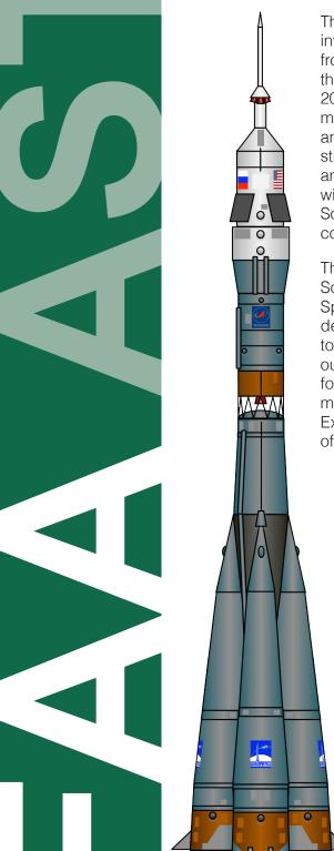
The Soyuz FG vehicle (11A511FG), introduced in 2001, is an improvement from the Soyuz U (11A511U) vehicle that was in service from 1973 to 2015. The improvements focused mainly on upgrades to the RD-108 and RD-107 engines. The vehicle still uses an analog control system, and it is anticipated that the vehicle will ultimately be replaced by the Soyuz 2 series, which has a digital control system.
