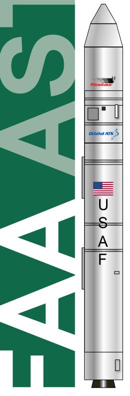
The Minotaur IV is an orbital launch vehicle offered by Orbital ATK. The vehicle is derived from the Peacekeeper intercontinental ballistic missile (ICBM).
