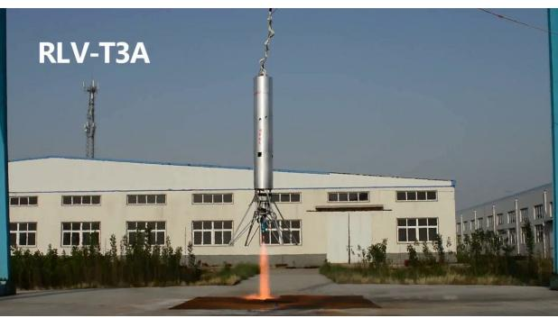
Link Space conducts a hover test in 2016 using a tethered testbed vehicle. (Source: Link Space)
