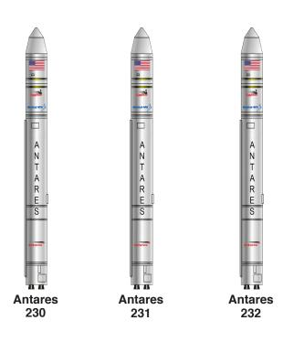
The Antares is offered in three variants. The first stage, which is common to all variants, is outfitted with a CASTOR 30XL solid motor upper stage. The vehicle can have no third stage, or an option between a Bi-Propellant Third Stage (BTS) or a STAR 48. The same fairing is used for all six versions.
