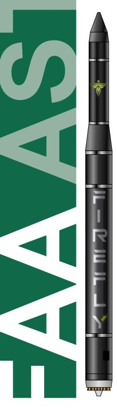
U.S.-based company Firefly Aerospace Inc. ("Firefly") plans to offer the Alpha launch vehicle to service the burgeoning small-satellite industry. Alpha is a two-stage vehicle, utilizing composite materials to create strong lightweight primary structures such as the airframe and propellant tanks.
