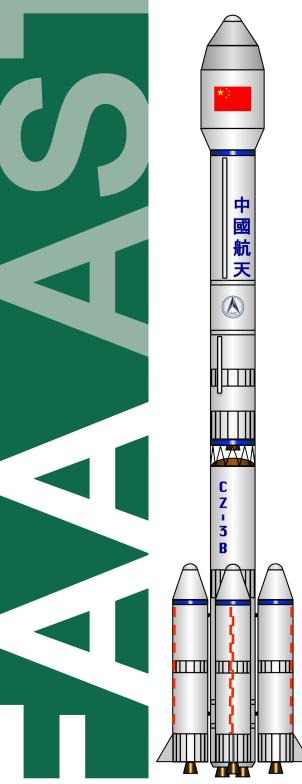
With a low Earth orbit (LEO) capacity of 12,000 kg (26,456 lb), the Long March 3B is currently China's most powerful launch vehicle. The vehicle is derived from the Long March 3A vehicle, with the key difference being that the Long March 3B uses four liquid boosters. The vehicle is primarily used for missions to a geostationary transfer orbit (GTO), but can be used for uncrewed science missions to the Moon (Chang'e-3).
