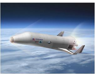
Northrop Grumman's subsidiary, Scaled Composites, is developing this team's XS-1 concept. The concept includes a clean-pad approach using a transporter erector launcher with minimal infrastructure and ground crews, highly autonomous flight operations, and horizontal landing and recovery on standard runways. Virgin Galactic would manage operational missions. (Source: Northrop Grumman)
