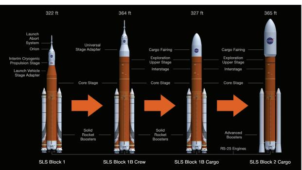
A NASA diagram showing the evolution of the Space Launch System. (Source: NASA)
