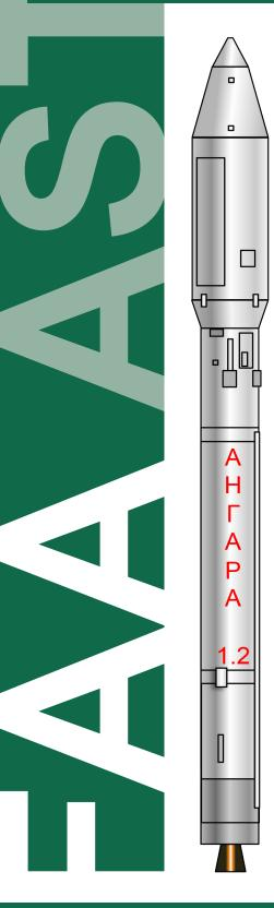
Russia's Angara series of launch vehicles is being developed by Khrunichev, designed to ultimately replace the Proton M and a variety of medium and small vehicles like Dnepr and Rockot. The Universal Rocket Module (URM-1) forms the modular core of every Angara vehicle.
