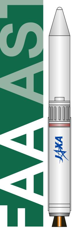
The Epsilon is a vehicle under development by the Japan Aerospace Exploration Agency (JAXA), derived from the Nissan-built M-V discontinued in 2006. The vehicle will be used to send small payloads to low Earth orbits and polar orbits. The first launch of Epsilon took place during 2013, successfully placing a small payload into low Earth orbit (LEO).
