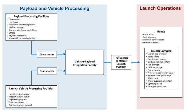
Figure 3. A typical arrangement for a launch site and range.
