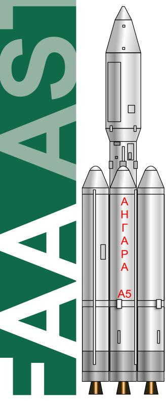
The Khrunichev State Research and Production Space Center has been developing the Angara series of vehicles to replace virtually all vehicles in service with the exception of the Soyuz. The Angara 1.2 is expected to replace the Rockot and Dnepr while the Angara A5 is expected to replace the Proton M within 5-7 years. The Universal Rocket Module (URM-1) forms the modular core of every Angara vehicle, with a URM-2 used as a second stage. A Breeze-M upper stage serves as an optional third stage.
