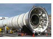
A 5-segment Solid Rocket Booster being prepared for ground test firing (Orbital ATK)
