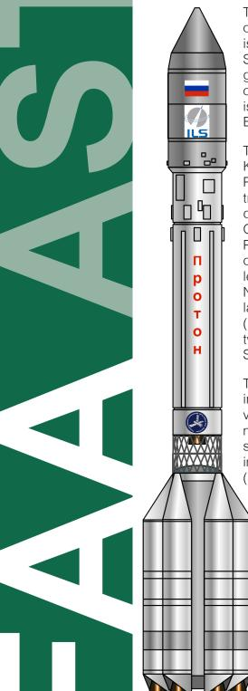
The Proton Medium, a 2-stage version of the venerable Proton M vehicle, is provided by International Launch Services (ILS) as a launch option for government and commercial operators of satellites in geosynchronous orbit. It is typically not used for missions to low Earth orbit (LEO).
