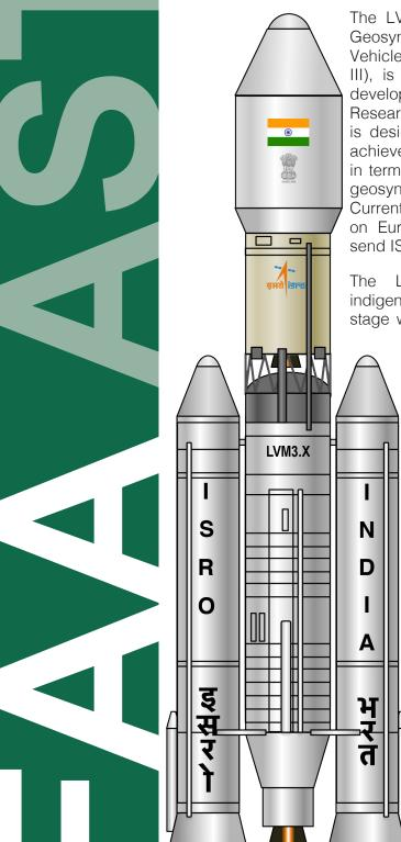
The LVM3, formally called the Geosynchronous Space Launch Vehicle Mark III (GSLV Mk III), is a launch vehicle being developed by the Indian Space Researc organization (ISRO). It is designed to enable India to achieve complete self reliance in terms of sending satellites to geosynchronous orbits (GEO). Currently, India largely depends on Europe's Ariane 5 ECA to send ISRO payloads to GEO.
