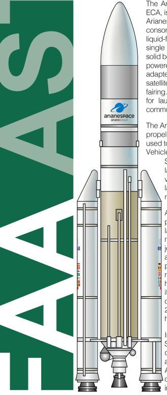
The Ariane 5, technically the Ariane 5 ECA, is the workhorse of France-based Arianespace, a European launch consortium. The Ariane 5 consists of a liquid-fueled core stage powered by a single Vulcain 2 engine, two strap-on solid boosters, a cryogenic upper stage powered by an HM7B engine, a payload adapter that can accommodate two satellites (called SYLDA), and a payload fairing. The Ariane 5 ECA is optimized for launches of two geosynchronous communications satellites.
