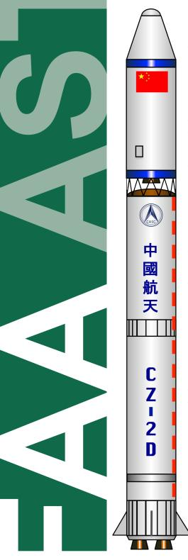
Primarily used to lift payloads to LEO and SSO, the 41-meter-tall, two-stage Long March 2D launch vehicle is part of the Long March 2 family of rockets. First launched from Jiuquan Satellite Launch Center in 1992, this Chinese launch vehicle has completed 25 successful launches. Two variants of the Long March 2D are known, and both are two-stage rockets that employ engines fueled by N<sub>2</sub>O<sub>4</sub>/UDMH.
