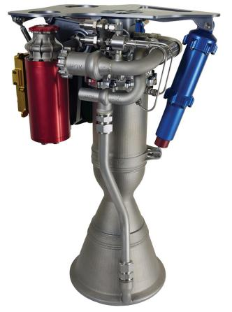
Rocket Lab's Rutherford engine. All its primary components are produced using additive manufacturing, or 3D printing. (Source: Rocket Lab)
