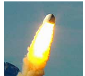
Blue Origin's Crew Capsule escape system test in October 2012.
