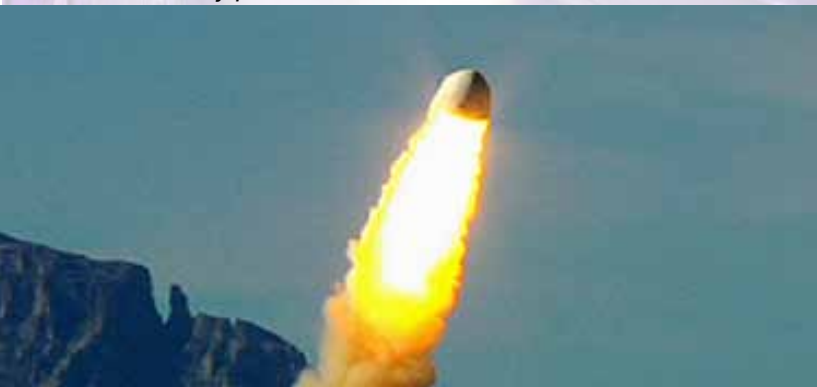
October 2012: Successful test of Blue Origin's crew capsule escape system, which reached an altitude of 703 meters and returned by parachute.
