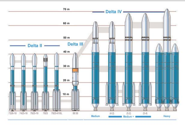
Figure 4: Delta Vehicle Lineage
