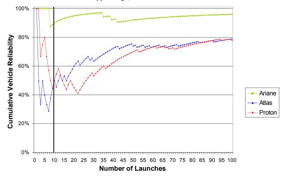
Figure 1: Cumulative Vehicle Reliability for the First 100 Launches
