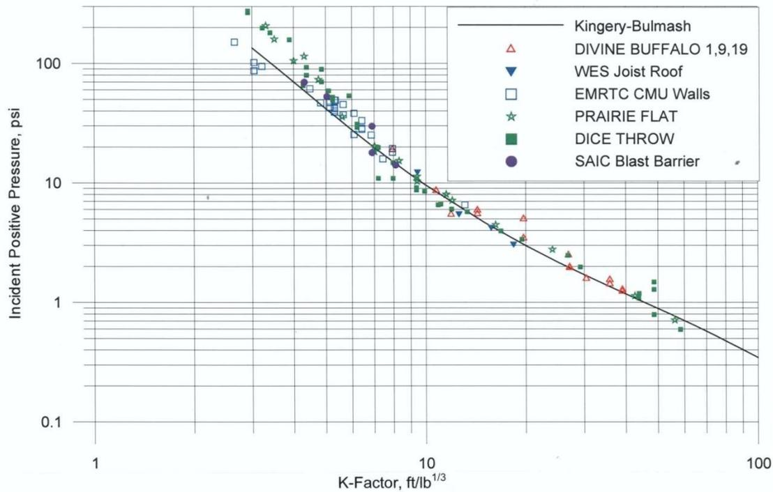
**Figure 1: Kingery-Bulmash Relationship with Blast Test Data Points**
