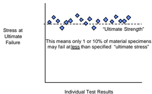
90 or 99% of Material Tests Must Pass at 95% Confidence Level
