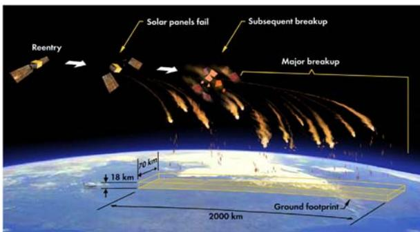
Figure 7. Dimensions of airspace affected by a spacecraft reentry event.
