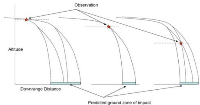
Figure 10. Illustration of effect of altitude of reentering object at observation on the length of the predicted impact zone.
