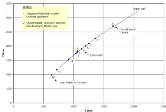
Figure 6. Ground distribution of debris after reentry breakup, Object 2.
