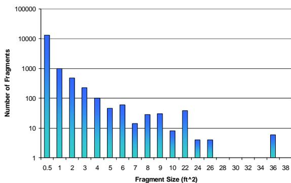
Figure 4. Size distribution of recovered Columbia Debris (note that x-axis is not uniform).
