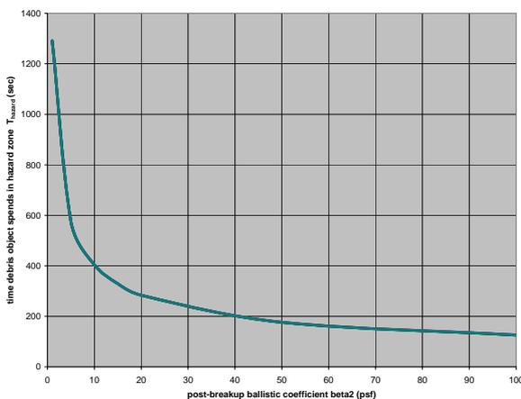
Figure 13. Time objects spend in hazard zone as a function of subsonic ballistic coefficient.
