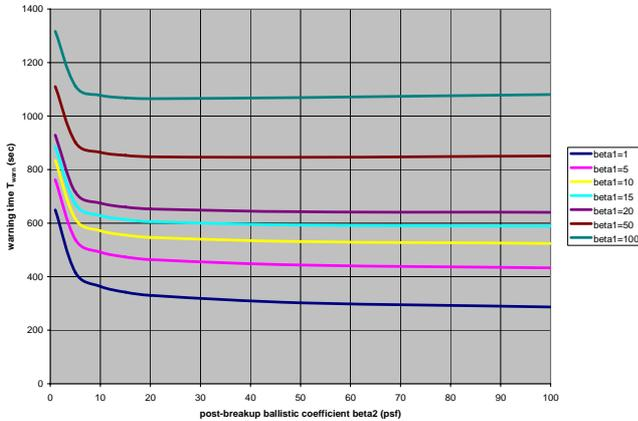
Figure 12. Time from breakup at 42nmi to 60,000 ft (hypersonic ballistic coefficients).
