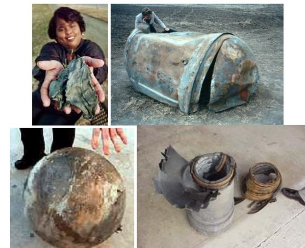
Figure 2. Debris from Delta II Second Stage reentry: from left: Lightweight fragment, propellant tank, sphere, thrust chamber. Photos courtesy Tulsa World (staff photo by Brandi Stafford), NASA, NASA, Aerojet, respectively).
