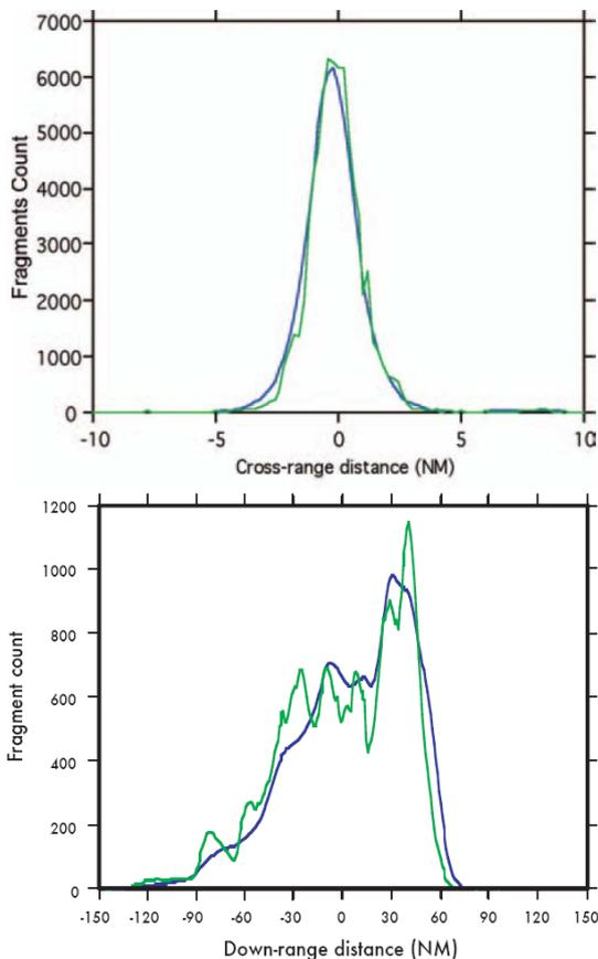
Figure 3. Downrange and crossrange distribution for debris from Columbia accident.
