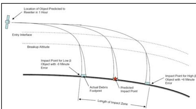
Figure 8. Possible downrange impact points from observation prior to breakup.
