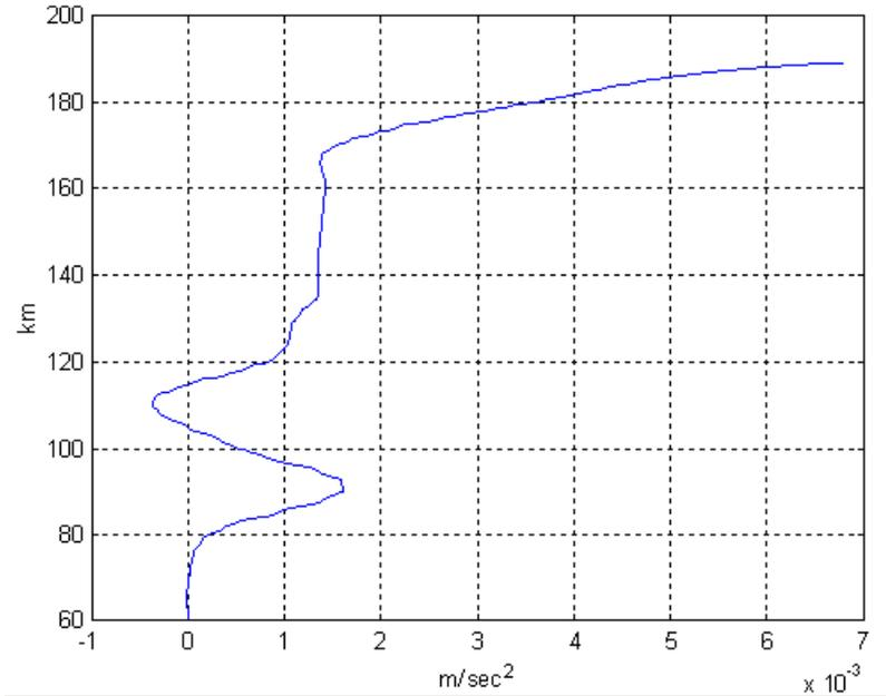
Figure 8. Ionosphere induced apparent acceleration
