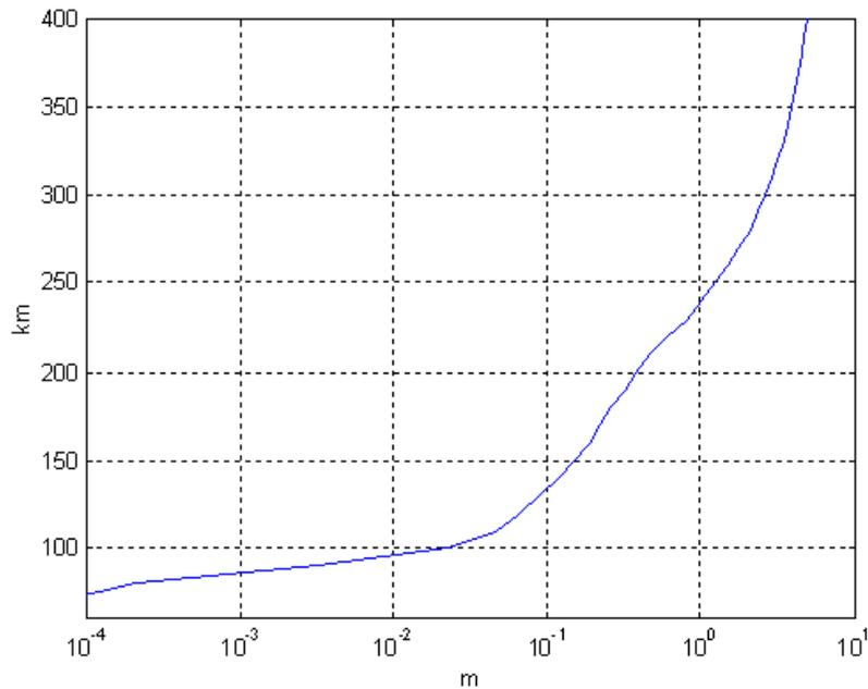
Figure 6. Difference in ionosphere delay between ground level and an altitude.
