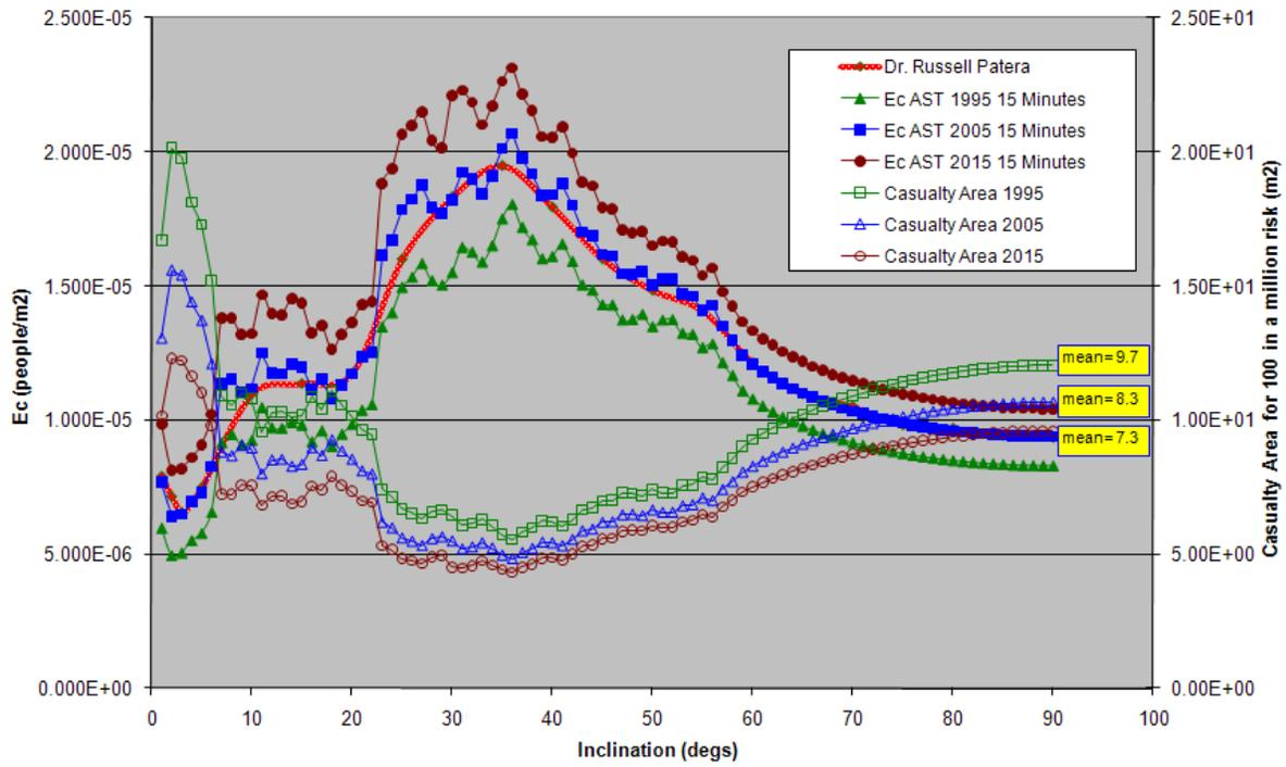
Figure 4. Random Reentry Collective Risk vs. Orbital Inclination
