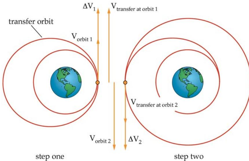
**Figure 4.1.5-5. Hohmann Transfer.** Step 1: The first burn or  $\Delta V$  of a Hohmann Transfer takes the spacecraft out of its initial, circular orbit and puts it in an elliptical, transfer orbit. Step 2: The second burn takes it from the transfer orbit and puts it in the final, circular orbit.
