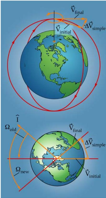
**Figure 4.1.5-9. Changing  $\Omega$ .** A simple plane change as a spacecraft crosses the pole in a polar orbit ( $i = 90^\circ$ ) will change only the right ascension of the ascending node,  $\Omega$ . Imagine the orbital plane pivoting about Earth's poles.
