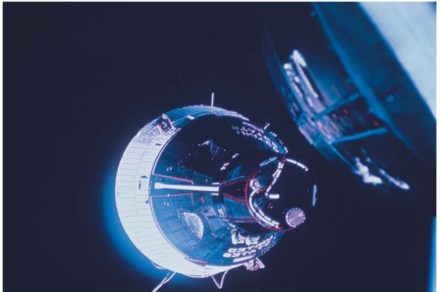
**Figure 4.1.5-2. The Gemini Program.** During the Gemini program in the 1960s, NASA engineers and astronauts developed the procedures for all orbital maneuvers needed for the complex Lunar missions. Here the Gemini 6A command module is rendezvousing with the Gemini 7 command module. (Courtesy of NASA/Johnson Space Center)
