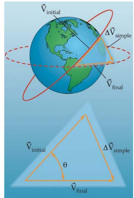
**Figure 4.1.5-8. Simple Plane Change.** A simple plane change affects only the direction and not the magnitude of the original velocity
