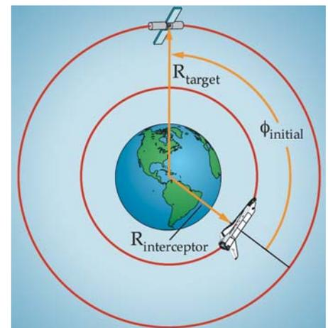
**Figure 4.1.5-13. Rendezvous Initial Condition.** At the start of the rendezvous problem, the target is some angle,  $\phi_{\text{initial}}$ , away from the interceptor.
