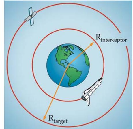
**Figure 4.1.5-11. The Rendezvous Problem.** The Space Shuttle commander must do a Hohmann Transfer at precisely the right moment to rendezvous with another spacecraft.
