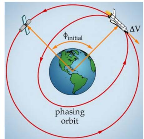
**Figure 4.1.5-14. Slow Down to Speed Up.** To catch another spacecraft ahead of it in the same orbit, an interceptor slows down, entering a smaller phasing orbit with a shorter period. This allows it to catch the target.
