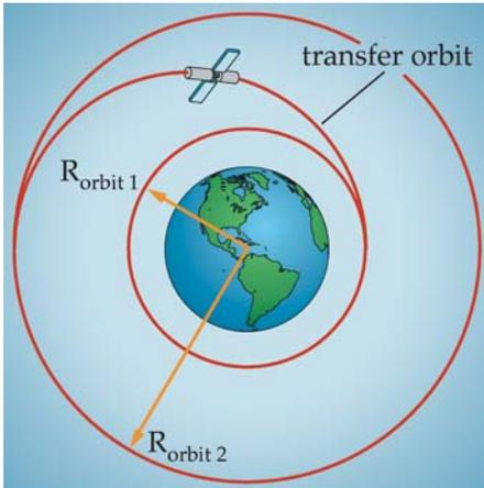
**Figure 4.1.5-4. Getting From One Orbit to Another.** The problem in orbital maneuvering is getting from orbit 1 to orbit 2. Here we see a spacecraft moving from a lower orbit to a higher one in a transfer orbit. If it doesn't perform the second  $\Delta V$  when it reaches orbit 2, it will remain in the transfer orbit.
