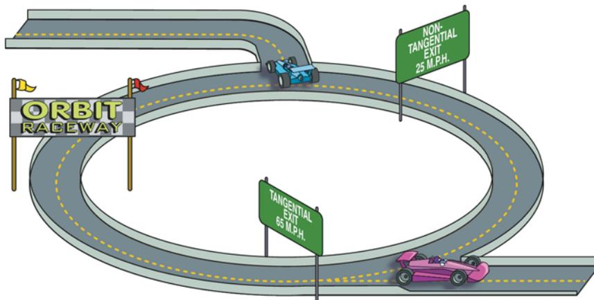
**Figure 4.1.5-3. Maneuvering.** One way to think about maneuvering in space is to imagine driving around a racetrack. Exiting at a sharp turn takes more effort than exiting tangentially.
