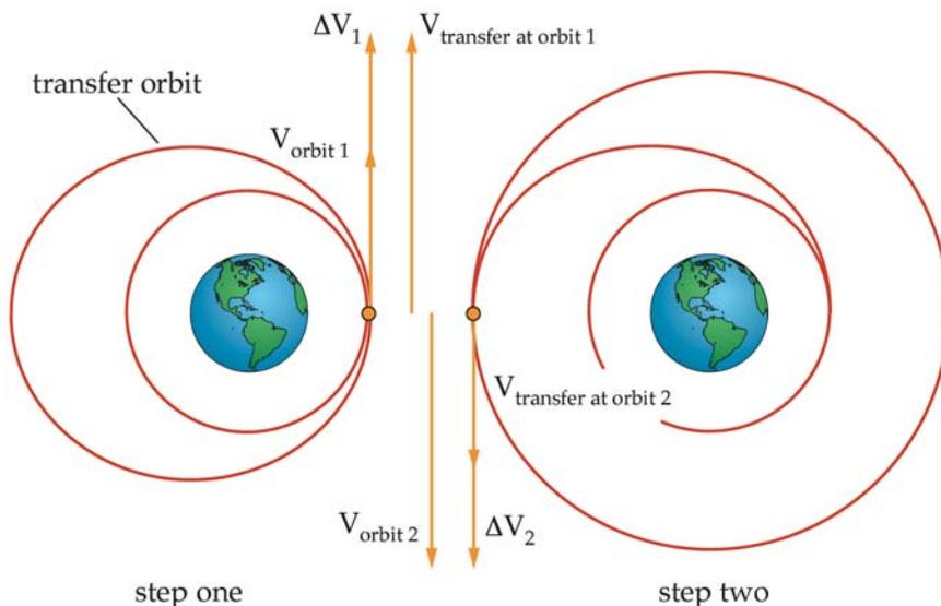
**Figure 4.1.5-6. Hohmann Transfer.** Step 1: The first burn or  $\Delta V$  of a Hohmann Transfer takes the spacecraft out of its initial, circular orbit and puts it in an elliptical, transfer orbit. Step 2: The second burn takes it from the transfer orbit and puts it in the final, circular orbit.
