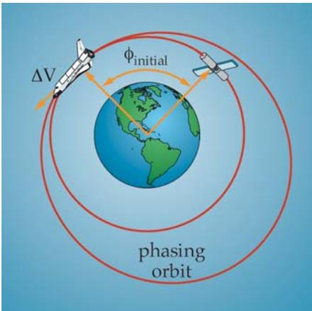
**Figure 4.1.5-15. Speed Up to Slow Down.** If the target is behind the interceptor in the same orbit, the interceptor must speed up to enter a higher, slower orbit, thereby allowing the target to catch up.
