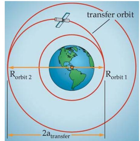
**Figure 4.1.5-7. Size of the Transfer Orbit.** The major axis of the transfer orbit equals the sum of the radii of the initial and final orbits.
