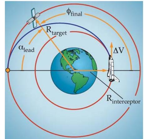
**Figure 4.1.5-12.  $\Delta V$  at the Right Time.** The first  $\Delta V$  of the rendezvous Hohmann Transfer starts when the interceptor is at an angle,  $\phi_{\text{final}}$ , from the target.
