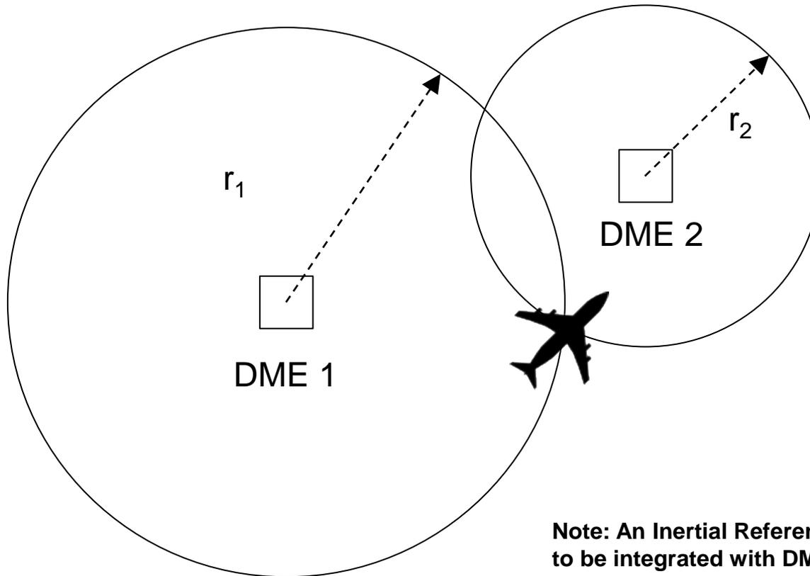
**Note: An Inertial Reference Unit (IRU) is required to be integrated with DME/DME in the U.S.)**
