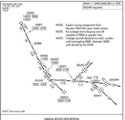
From KIDDZ on track 152° to cross SNIFY at 12000 and at 270K, then on track 152° to QTRBK, then on track 150° to cross RVEEE at or above 11000, then on track 147° to cross AAHZZ at 10000, then on track 148° to cross GLUVR at or above 9000 and at 240K.
