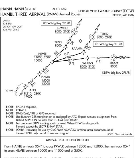
LANDING RUNWAY 21L/R: From HEMIE on track 084° to RAAMM, then on track 037° to cross TBRRD at 8000 and at 210K, then on track 036°. Expect RADAR vectors to final approach course.
