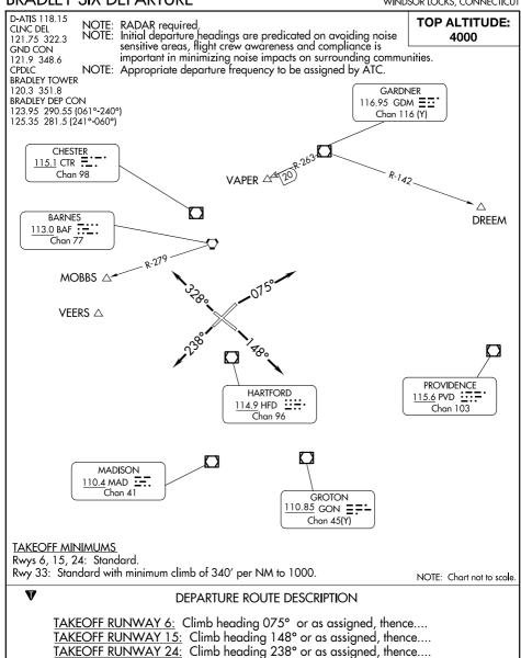
TAKEOFF RUNWAY 24: Climb heading 238° or as assigned, thence.... TAKEOFF RUNWAY 33: Climb heading 328° or as assigned, thence....
