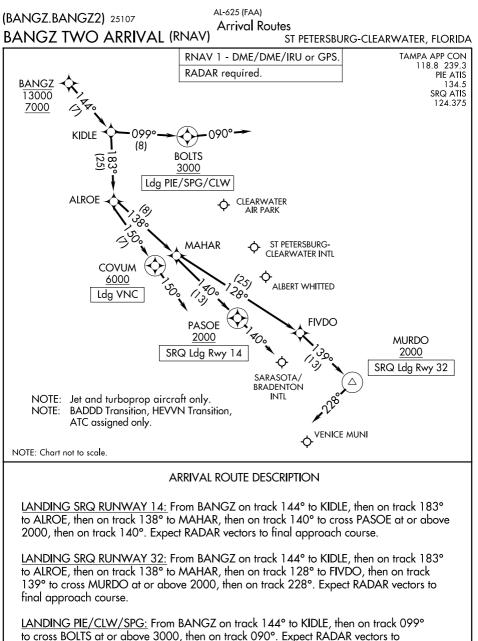
LANDING VNC: From BANGZ on track 144° to KIDLE, then on track 183° to ALROE, then on track 150° to cross COVUM at or above 6000, then on track 150°. Expect RADAR vectors to final approach course.
