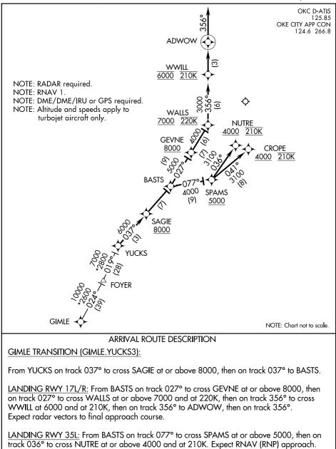
LANDING RWY 35R: From BASTS on track 077° to cross SPAMS at or above 5000, then on track 041° to cross CROPE at or above 4000 and at 210K. Expect RNAV (RNP) approach.
