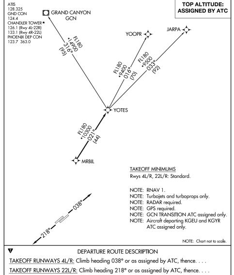
....expect RADAR vectors to MRBIL, then on track 021° to YOTES, then on (transition). Maintain ATC assigned altitude, expect filed altitude 3 minutes after departure.
