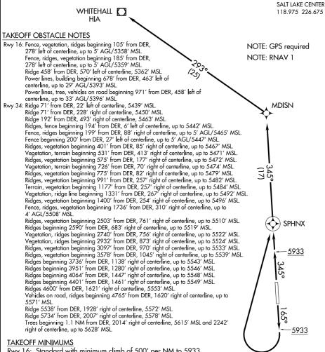
Rwy 16: Standard with minimum climb of 500' per NM to 5933, then minimum climb of 288' per NM to 8800.
