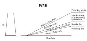
CAUTION: When viewing the pulsating visual approach slope indicators in the pulsating white or pulsating red sectors, it is possible to mistake this lighting aid for another aircraft or a ground vehicle. Pilots should exercise caution when using this type of system.
