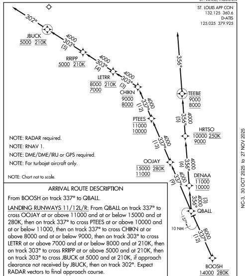
LANDING RUNWAYS 29/30L/R: From QBALL on track 356° to cross DENAA at or above 10000 and at or below 11000, then on track 356° to cross HRTSO at or above 9000 and at or below 10000 and at 250K, then on track 356° to cross TEEBE at or above 8000 and at or below 9000, then via assigned instrument approach procedure. If approach clearance not received by TEEBE, then on track 356°, expect RADAR vectors to final approach course.
