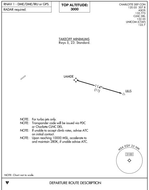
Climb on heading assigned by ATC, on RADAR vectors to LAMDE, then on depicted route to LILLS. Maintain 3000. Expect clearance to filed altitude within 10 minutes after departure.
