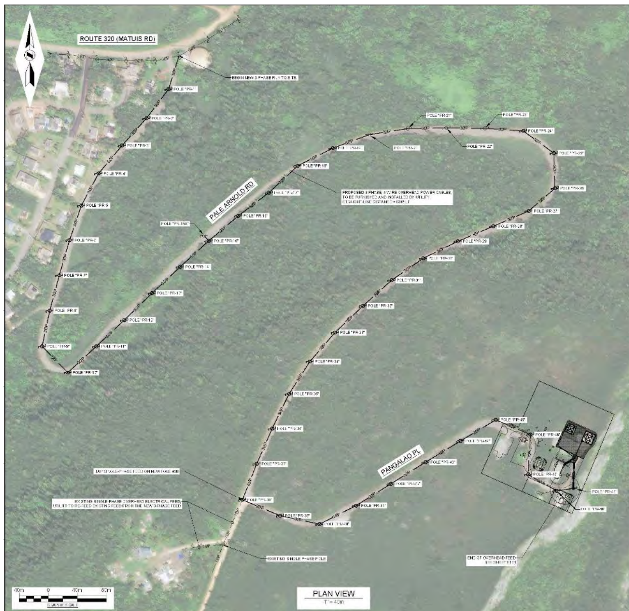
Figure 2-2 Aerial image showing the proposed electrical line distribution (ELD) upgrade along the existing utility corridor, including the locations of proposed typhoon-resistant concrete power poles. Construction Drawings, CUSA Consulting. 4/4/2025.
