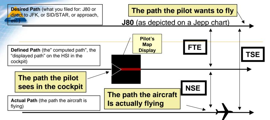
The **Navigation System Error** (NSE) is the difference between the <u>"actual" path</u> of an aircraft and its <u>"defined"</u> (displayed or computed) <u>path.</u> The difference between the <u>"desired path"</u> and the <u>"defined path"</u> is called **Flight Technical Error** (FTE). The vector sum of NSE and FTE is **Total System Error** (TSE).
