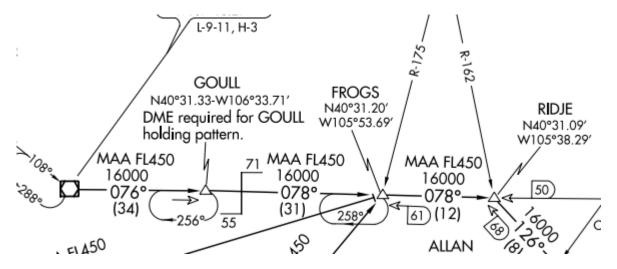
Holding patterns have been established at GOULL and FROGS intersections. Neither holding pattern is charted with a distance, leading to the assumption that both follow the aforementioned
