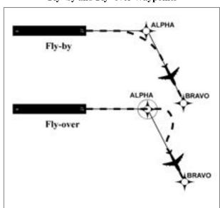
FIG 1-2-2 Fly-by and Fly-over Waypoints
