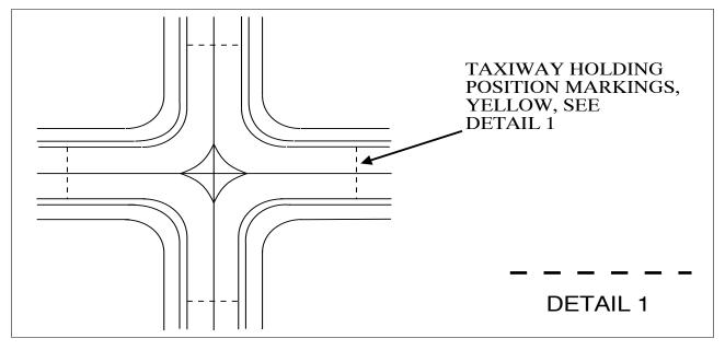
FIG 2-3-18 Vehicle Roadway Markings
