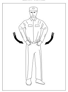
FIG 4-3-22 Cut Engines
