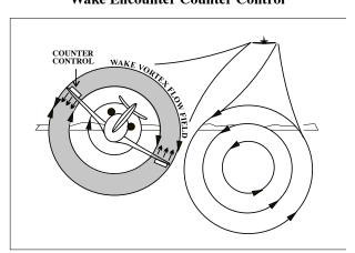
FIG 7-4-2 Wake Encounter Counter Control
