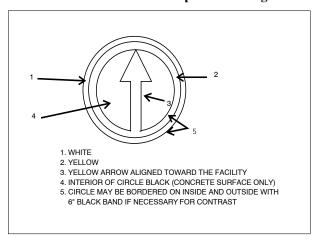
FIG 2-3-21 Nonmovement Area Boundary Markings
